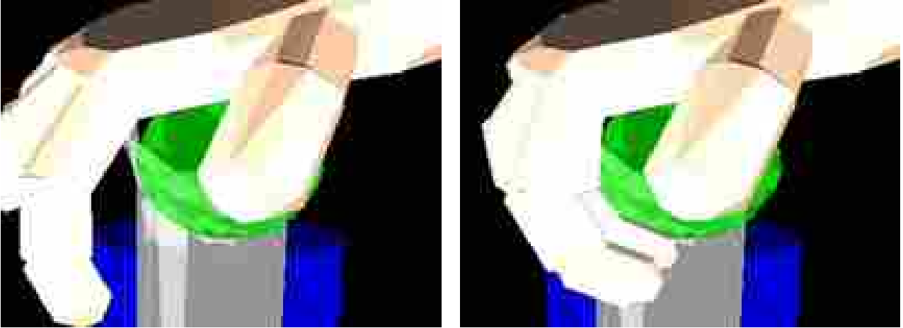
Figure 9: Natural grasping is basically a minimization problem for the flex vector under the constraint that finger-joints (and palm) must not penetrate the object.
