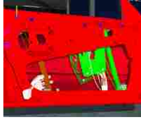
Figure 5.9: The window regulator has to be installed with two hands; the “ghost” paradigm signals collisions.
