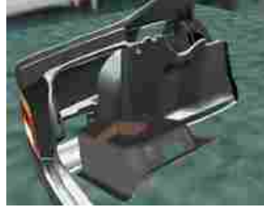
Figure 5.12: Inverse kinematics is needed for "door-like" behavior of parts.
