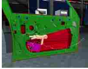
Figure 5.14: During assembly, the path of any part can be recorded, edited, and stored in the PDM system.
