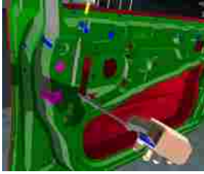
Figure 5.8: Tools snap onto screws and are constrained. Also, they are placed automatically at an ergonomic position within the hand by the system.
