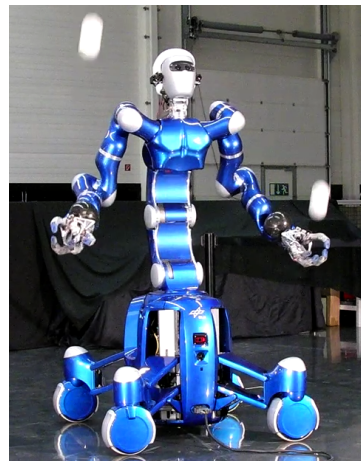
Fig. 1. Rollin’ Justin [6] catching two simultaneously thrown balls. The mobile humanoid consists of an omnidirectional platform with variable footprint and an upper body with 19 active DOF, built from two DLR-LWR-III arms [7] with 7 DOF, a torso with 3 (+1 passive) DOF and a neck with 2 DOF, and is equipped with two 12 DOF DLR-Hand-II [8]. The system operates completely wirelessly using only onboard sensing (see Sec. V). Weight: upper body 45 kg; mobile base 150 kg.
