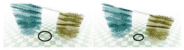
Fig. 4. **6-DOF SLAM map.** before and after closing the large loop (between the two building on the ground level) over all n = 106657 features. The black ellipses show the region where the loop is closed. The whole mapping process can be seen as 3D animation accompanying the article.
