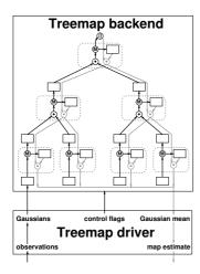
Fig. 2. Data flow between treemap backend and driver. The driver adds new leaves computed from new observations to the tree (here shown for the leftmost leaf). It further sets flags *invalid*, *integrable* for leaves as well as *marginalizable*, *sparsifyable* for random variables to control approximations conducted by the backend. In turn it receives the Gaussians mean and converts it into a map estimate.
