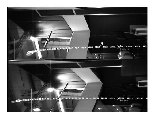
dictions as a function of time. One can observe the high accuracy (< 10cm) achieved even for the early predictions, with the major error occurring in the direction of the throw (x-axis in the figure). Figure 8 shows the throw as seen by the cameras. Overlayed is a early prediction of the trajectory.
