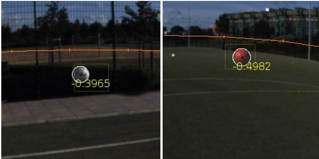
Figure 20: Correctly detected start balls with displayed (negative) error values
