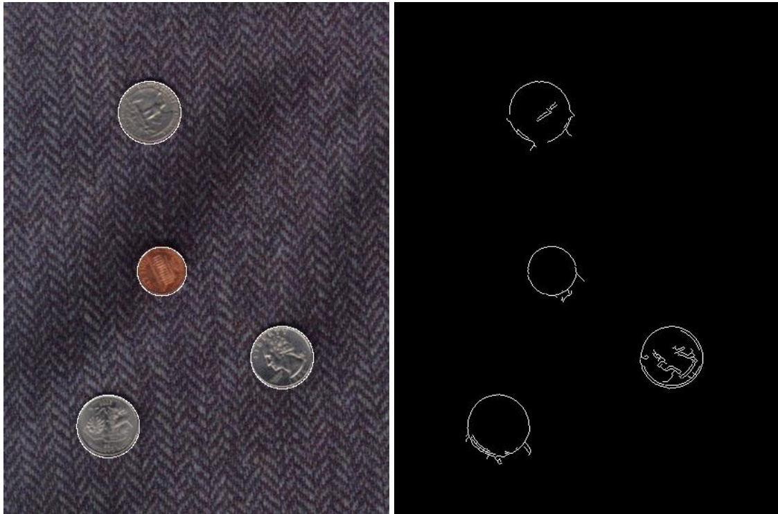
Figure 9: Source image (left), Standard Sobel image (right)
