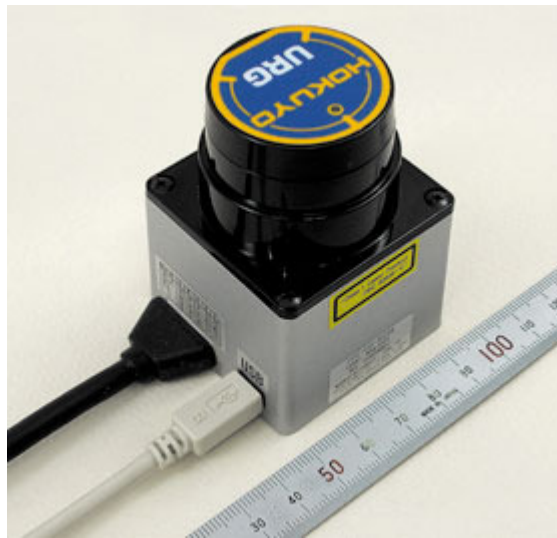
Abbildung 13: Laserscanner Hokuyo URG-04LX[24]
