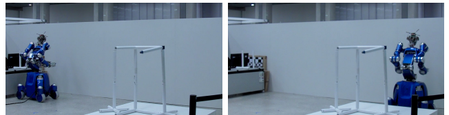
Fig. 4. For the experiment fusing Kinect depth data with odometry, Justin drives 4 m from the start pose (left) to the end pose (right) and back for 8 consecutive round trips per multi-wall-* dataset.
