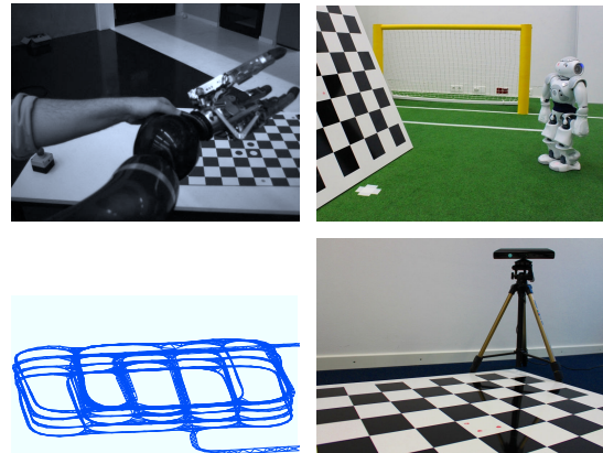
Fig. 1. Diverse problems solved with MTKM (top left to bottom right): Hand-eye, stereo and IMU calibration on a humanoid service robot, vertical stereo calibration on a humanoid soccer robot, 3D pose adjustment on the parking garage data set [21], and RGB-D and accelerometer calibration.
