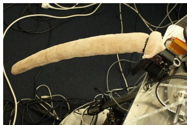
Figure 5-7: The attached tail. A cable binder was added after the coating fabric started to move outwards because of the motions.
