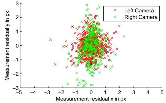
Fig. 3. Measurement residuals of left and right camera measurements.
