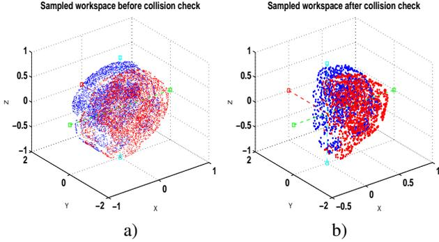
Fig. 2. The pose cloud obtained by the first stage of the active calibration algorithm used for experimentation. Blue markers belong to left arm and red markers to right arm. **a)** The pose cloud before checking for collisions. **b)** The remaining pose cloud after checking for collisions.
