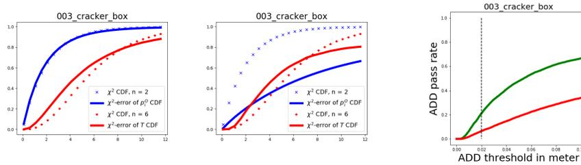
**Fig. 6.** Cumulative  $\chi^2$  curves on training (left) and test images (right). Solid lines show the measured curves for points and poses resp. The dotted lines show the theoretical curves, corresponding to perfectly correct posterior distributions.
