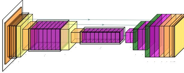
**Fig. 3.** CNN layers, where outputs are ordered according to Fig. 1: Shades from yellow to orange denote  $1 \times 1$ ,  $3 \times 3$  or  $5 \times 5$  convolutions; magenta, pairs of  $1 \times 1$  followed by  $3 \times 3$  convolutions; green, upsampling; blue, global pool and fully connected layers. All layers with trainable weights are followed by SELU [7] units. Output layers have no activation. For further details see <https://github.com/JesseRK/6D-UI-CNN-Output>.
