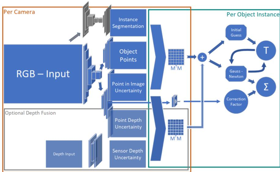
**Fig. 1.** Proposed architecture overview (cf. Section 3): CNNs take the image and optionally depth data and provide per-pixel instance segmentation, object points and uncertainties, as well as a per-object overall uncertainty correction factor (Section 4). This data is aggregated into a  $13 \times 13$  matrix  $M^T M$  and fused by a gPnP algorithm (Section 5) to a pose estimate  $T$  with covariance  $\Sigma$ .
