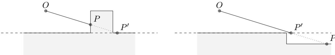
Figure 10.12: Positive obstacles (left) and negative obstacles (right) in GEM. The actual range measured is  $r_a = |\overline{OP}|$  while a range of  $r_e = |\overline{OP}'|$  was expected assuming there is nothing but the ground plane (dashed line). Obviously, anything beyond  $\min(r_a, r_e)$  must be considered as no longer drivable.
