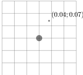
Figure 10.2: The local obstacle map is represented as a grid with the robot (large dot) at its center. Points are mapped into the grid through division by the cell side length and integer rounding. In this example the side length of cells is 0.05m.
