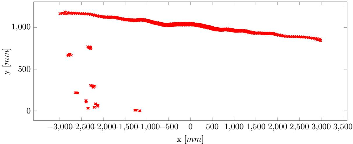
Figure 6.5: 40 consecutive raw ROD4plus scans showing the intersection with the ground plane in an indoor setting. Note the different scale on the two axes. The outliers are caused by table and chair legs.
