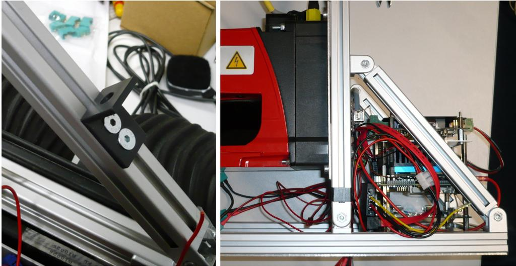
Figure 4.5: **Left:** A custom-built antenna mount allows for attaching the WiFi antenna to the frame and takes care of insulation. **Right:** Side view of the PC/104 stack, the vertically mounted SSD on the base plate, and the STM32 board (USB-A connector).
