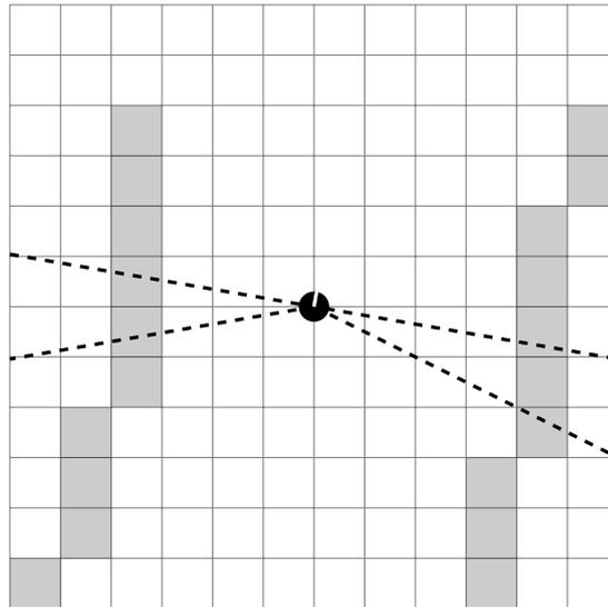
Figure 9.6: The “beams” of the virtual range sensors used to detect path boundaries are illustrated by the four dashed lines. The first obstacle cell intersected by each line determines the range measurement. Note that in the actual implementation the grid has a higher resolution and that the virtual sensor beams are rasterized using the supercover line approach from [section 11.3.3](#) on [page 113](#).
