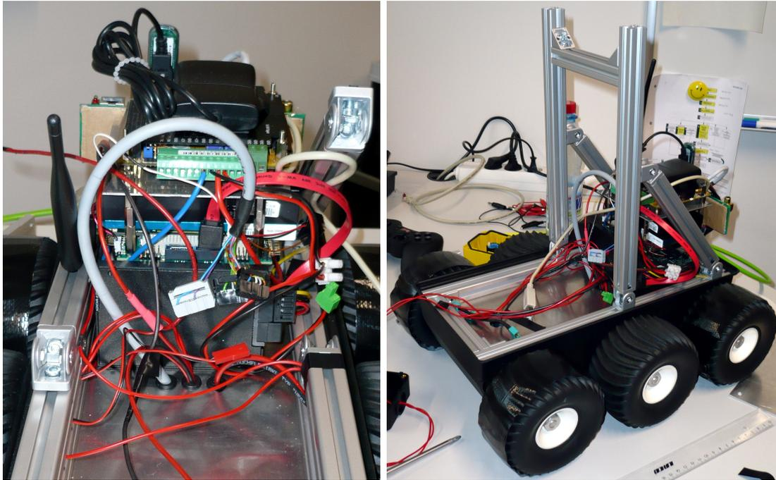
Figure 4.7: **Left:** With the laser range finder removed the grommets protecting the cables that pass through the base plate and the solid state disk (SSD) right behind them are clearly visible. **Right:** Shorter aluminium profiles have been installed to lower the center of gravity.
