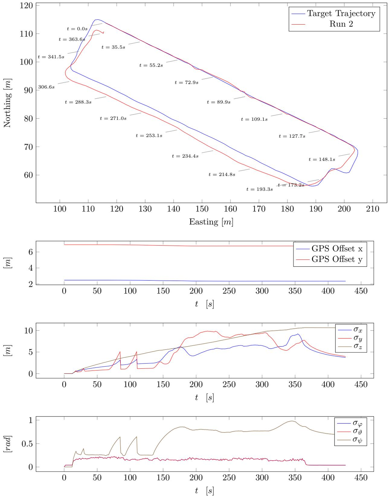
Figure 12.13: UKF position estimates with GPS and path boundary measurements enabled. Again,  $\sigma_\varphi$  and  $\sigma_\theta$  overlap.
