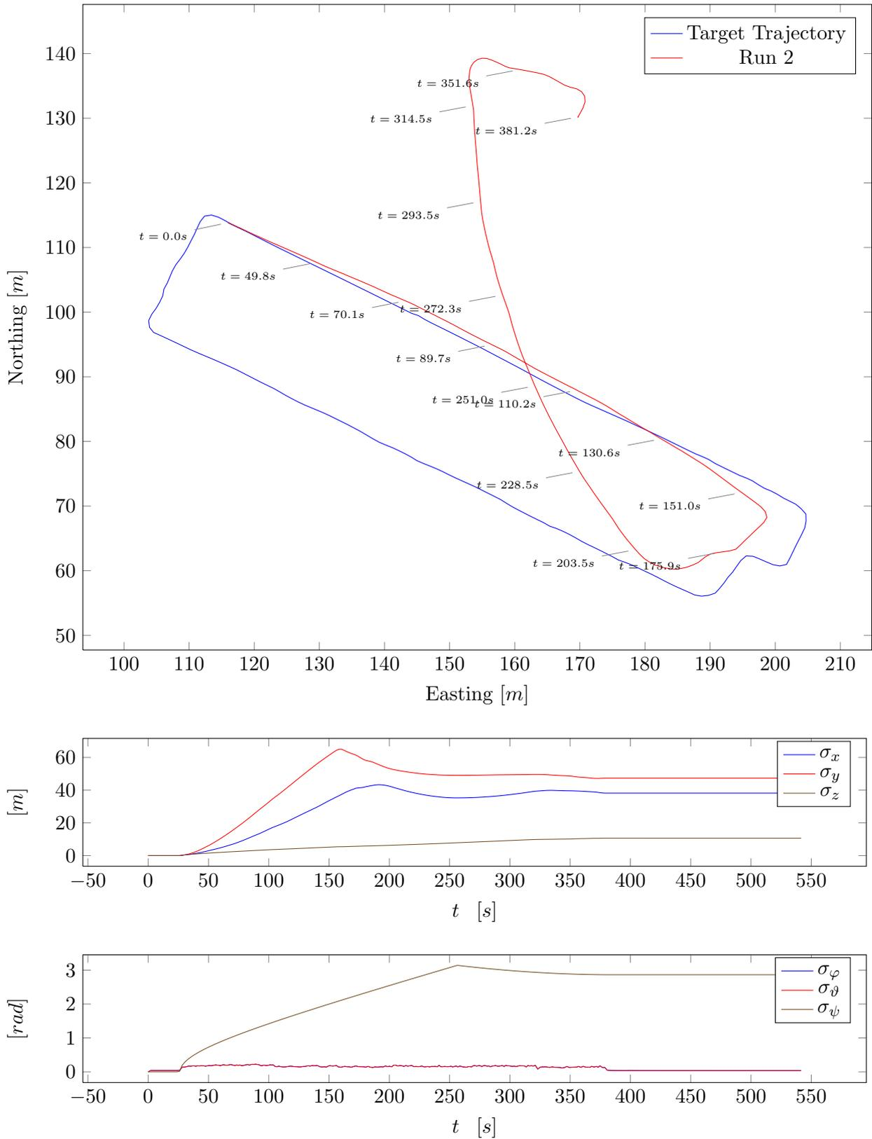
Figure 12.6: UKF position estimates with GPS and magnetometer measurements disabled. Note that, on the scale of the graph,  $\sigma_\phi$  and  $\sigma_\theta$  overlap as both are dominated by the same accelerometer measurements.
