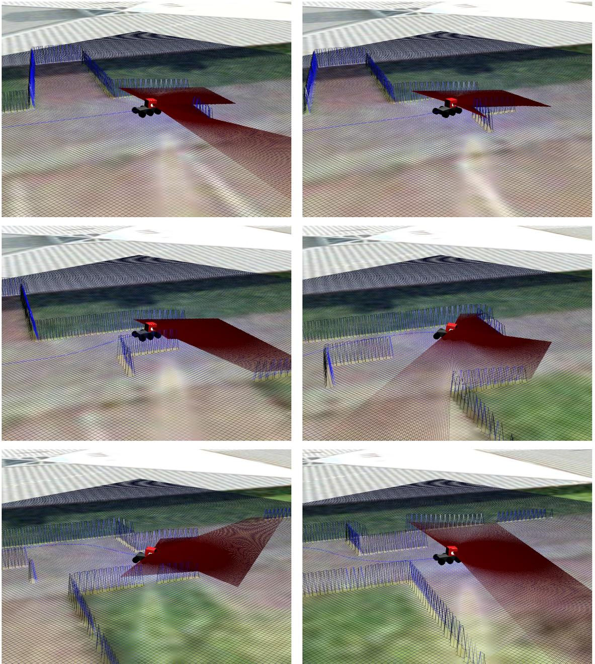
Figure 12.3: A sequence of visualization screenshots (top-left to bottom-right) showing the simulated robot as it successfully negotiates the two test obstacles.
