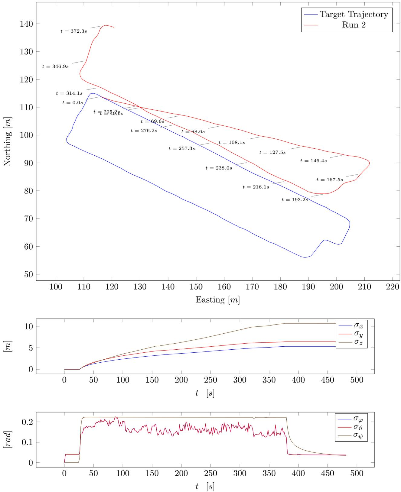
Figure 12.7: UKF position estimates with magnetometer measurements enabled and GPS disabled. Again,  $\sigma_\varphi$  and  $\sigma_\theta$  overlap.
