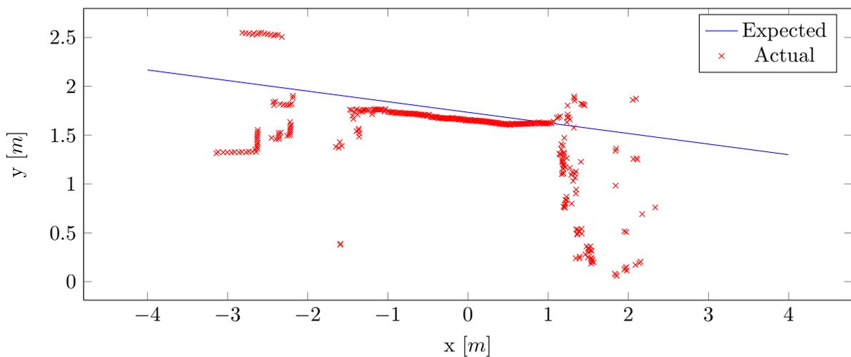
Figure 10.11: Expected ground plane intersection vs. actual laser range scan endpoints in an outdoor setting. The plot shows the scan plane.
