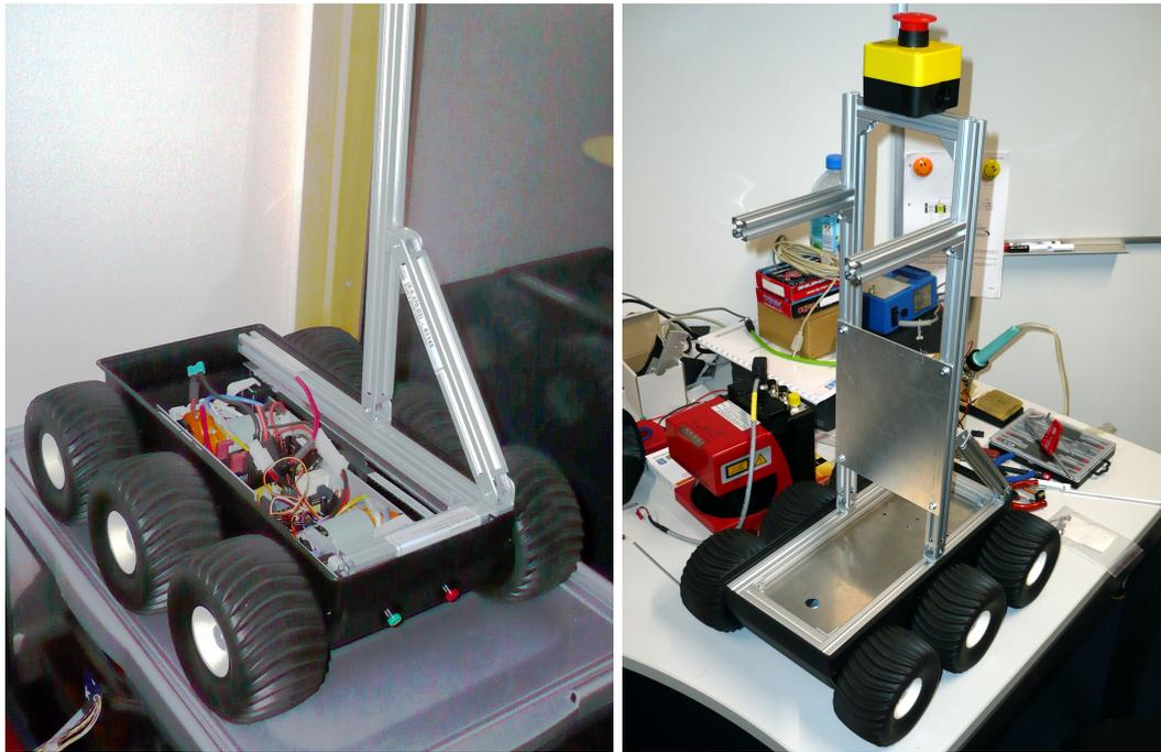
Figure 4.2: **Left:** The frame fits exactly into the upper part of the plastics chassis. **Right:** Of the original upper assembly only the base plate is re-used in the construction of the new frame.
