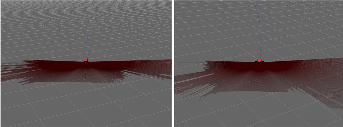
Figure 10.9: The visualization results that motivated the development of GEM. In front of the robot the range scans stem from hitting the ground on the drivable path. A human observer can easily distinguish range scans originating from positive or negative obstacles from these.
