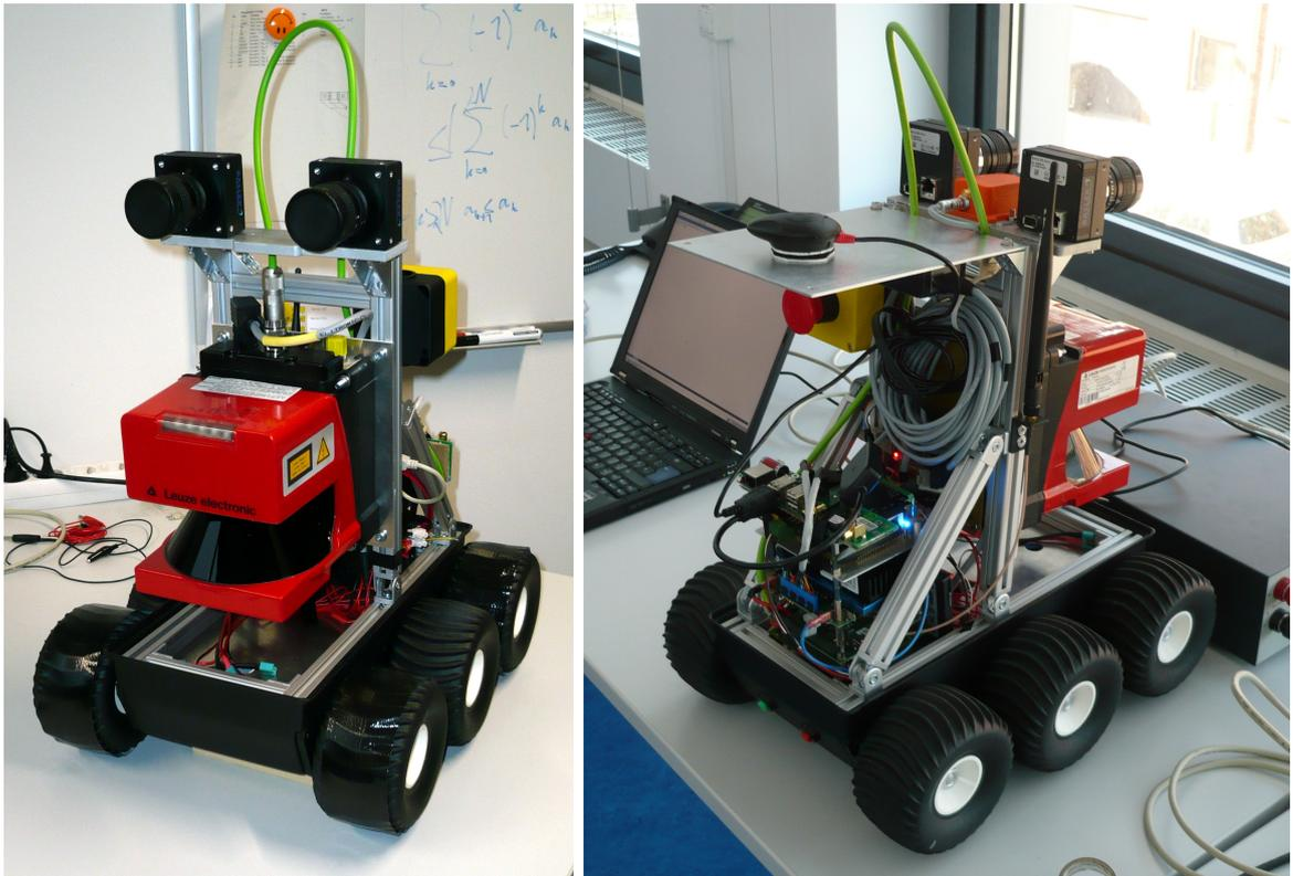
Figure 4.8: **Left:** The stereo-camera/IMU sensor head is mounted for the first time. Note the missing IMU. **Right:** Rear view of the SAMSMobil in its final configuration with all sensors (including the XSens IMU and the new Navilock GPS receiver).
