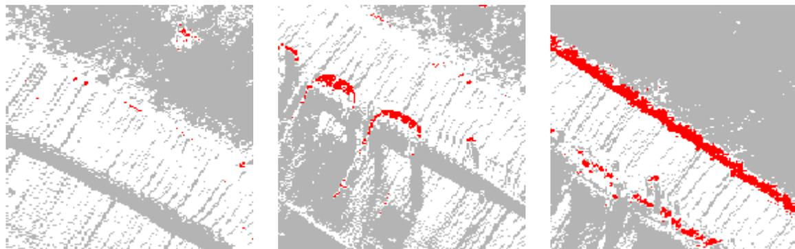
(a) Neither most of the patch of grass (above) nor the curb (below the path) are detected as obstacles.
