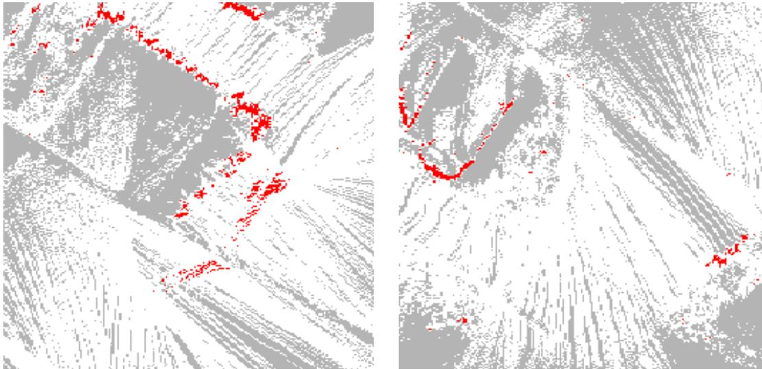
(a) Part of the ramp from the sidewalk (top) onto the road (bottom) is incorrectly detected as obstacles.
