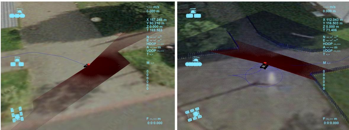
Figure 5.3: Visualization of the simulated robot pose and laser range scans (left) and additionally with the local map generated by the mapper (right).
