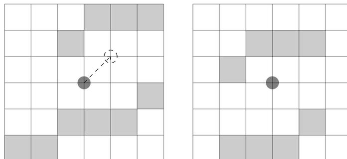
Figure 10.3: In a simplistic grid implementation previously entered obstacles (left) need to be moved to retain their relative position if the robot position changes (right).
