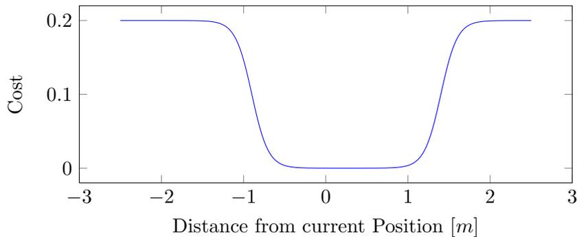
Figure 11.4: Valley function with sensed path boundaries at -1 m and 1.5 m relative to the current position perpendicular to the path.
