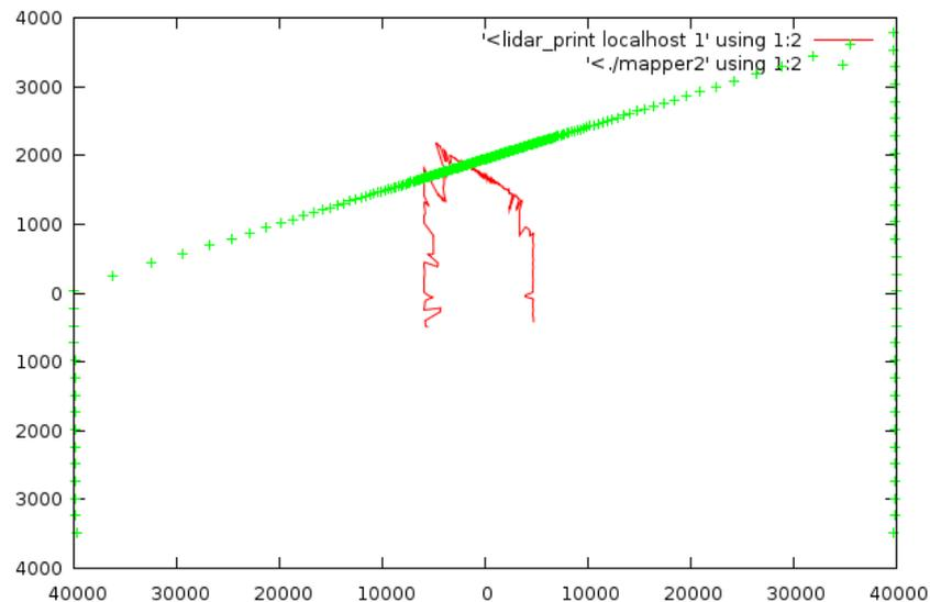
Figure 7.6: Assuming a pure translation for LIDAR2IMU the simulated range scan (green crosses) does not match the actual range scan (red line). The plot shows the scan plane (both axes in mm).
