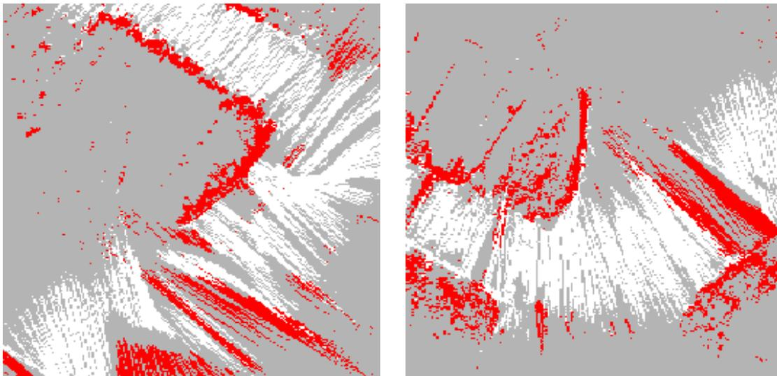
(a) The ramp from the sidewalk (top) onto the road (bottom) is detected as drivable. Both sides of the gutter are not.
