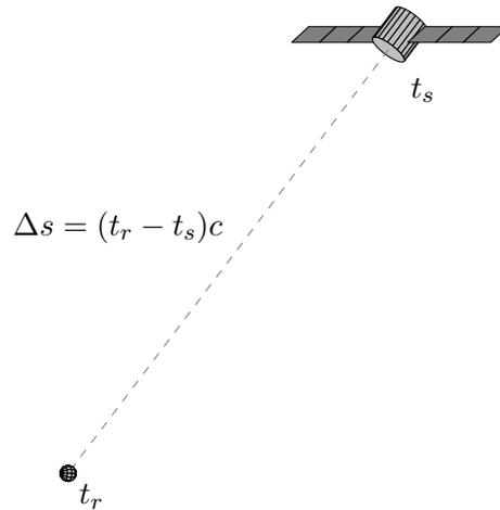
Figure 6.1: Determining range from time of flight in GPS.
