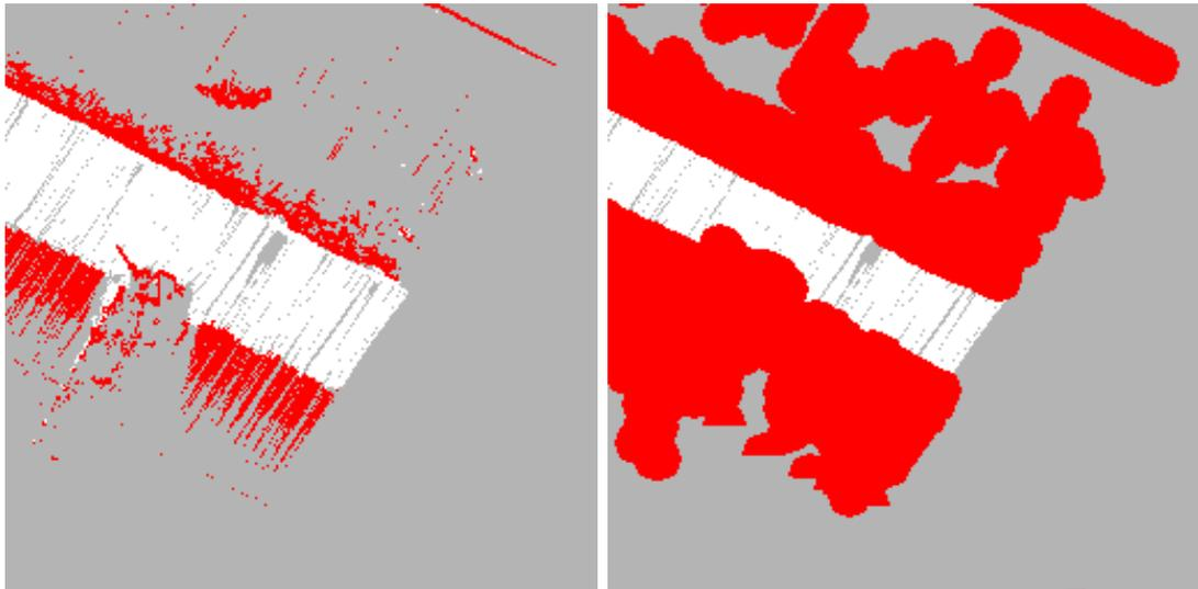
Figure 11.2: The local obstacle map before (left) and after obstacle extrusion (right).
