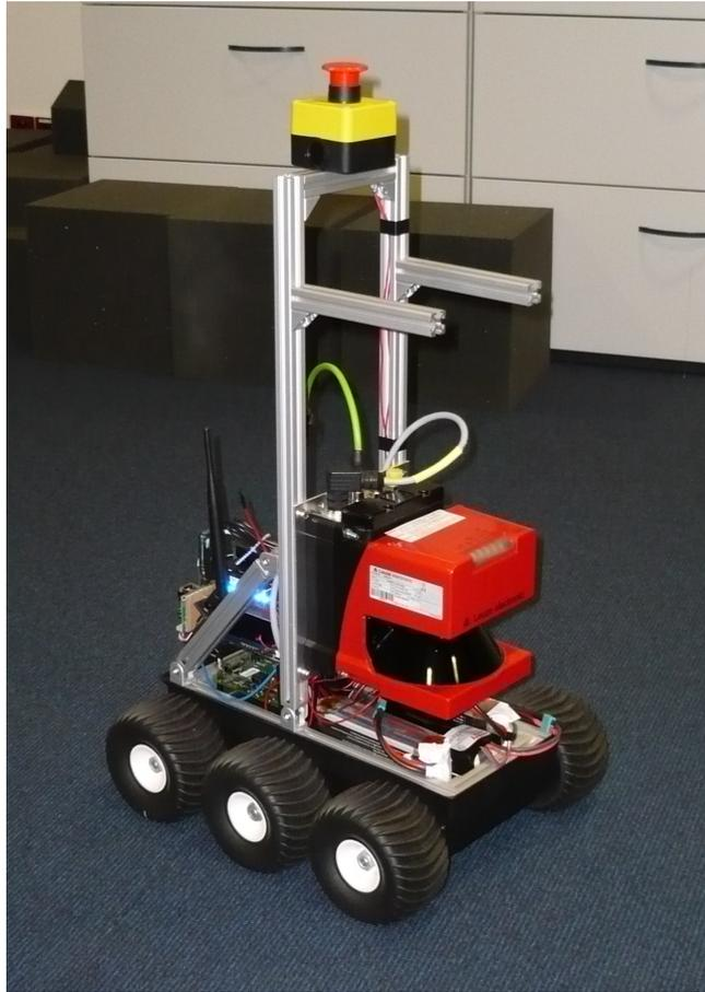
Figure 4.6: One of the first test runs with the rebuilt SAMSMobil. Note the battery packs below the laser range finder.
