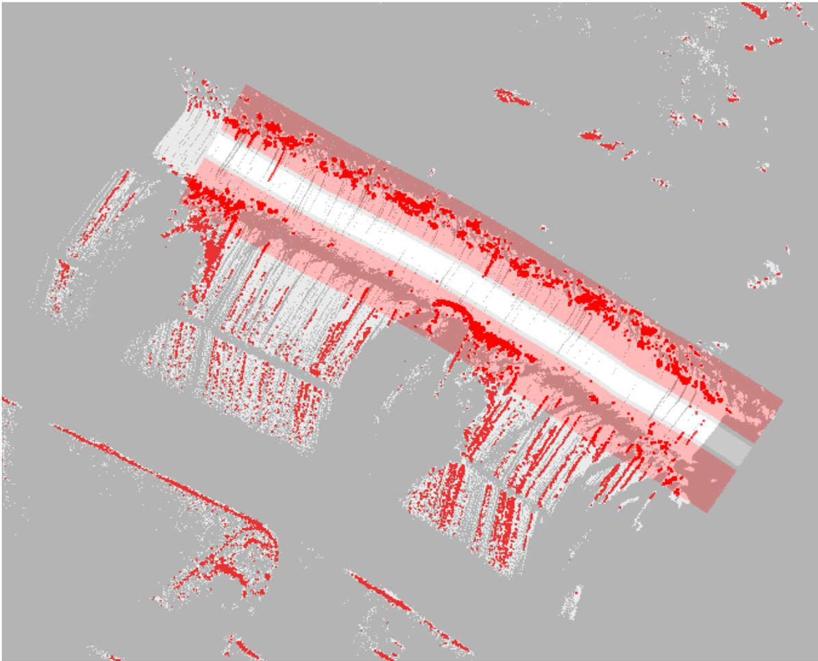
Figure 10.6: Automatic labeling of the grid cell drivability based on log data. The robot drove from the lower-right corner to the upper-left corner in the map. The white stretch is labeled as drivable because it was traversed by the robot. One stretch to the left and one to the right are assumed to correspond with the path and thus marked as non-drivable. All other cells are ignored in the machine learning process.
