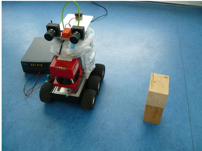
Figure 7.1: Laser range finder calibration setup
