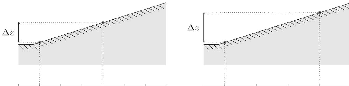
Figure 10.8: The classification of a ramp changes depending on the chosen grid cell size in PTA. The same gradient that is classified as drivable with a small cell size (left) is classified as an obstacle if the cell size is larger (right).
