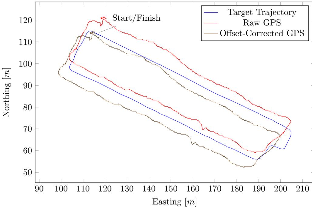
Figure 12.9: Raw vs. offset-corrected GPS. The offset correction compensates for a constant offset determined at the known initial position.
