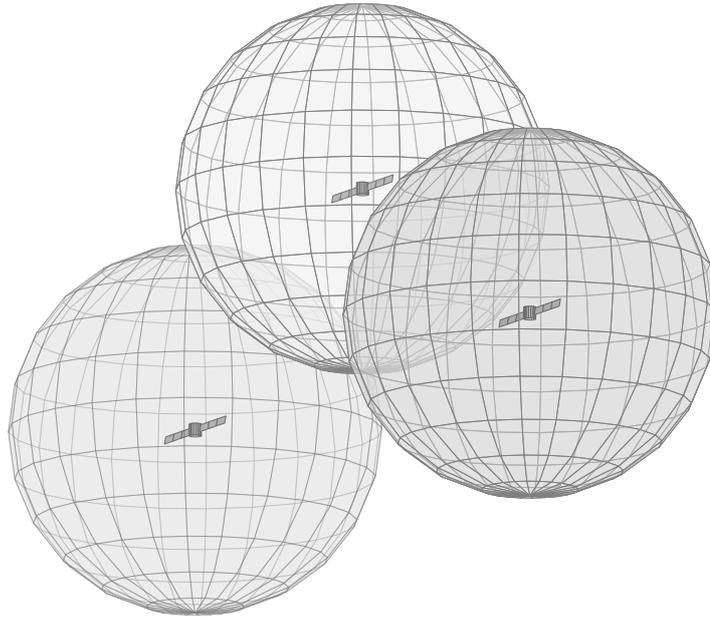
Figure 6.2: Positioning with pseudoranges from three GPS satellites. The pseudoranges determine the radius of each sphere. The positioning solution lies (approximately) where the three spheres intersect.
