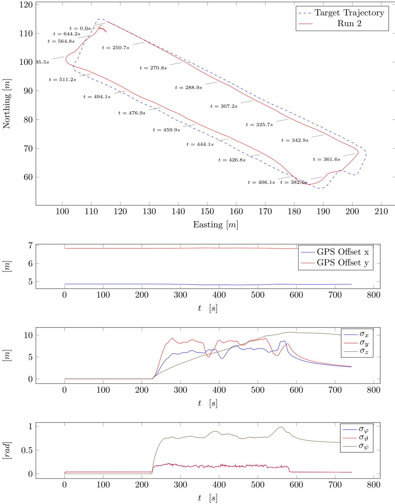
Figure 12.14: UKF position estimates with GPS projected onto the path. Again,  $\sigma_\varphi$  and  $\sigma_\theta$  overlap.
