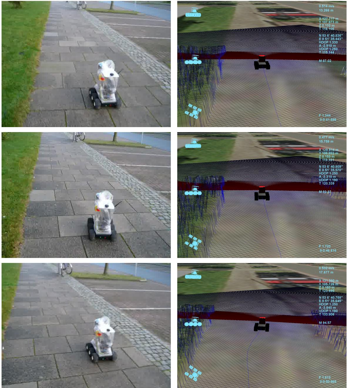
Figure 12.22: The SAMSMobil under autonomous control by the complete software stack in the 43 m test run. The real robot is shown on the left, its internal state belief and the obstacle map on the right, first shortly after the start of the test track (top), then while initiating a path centering response (middle). and after completing it (bottom).
