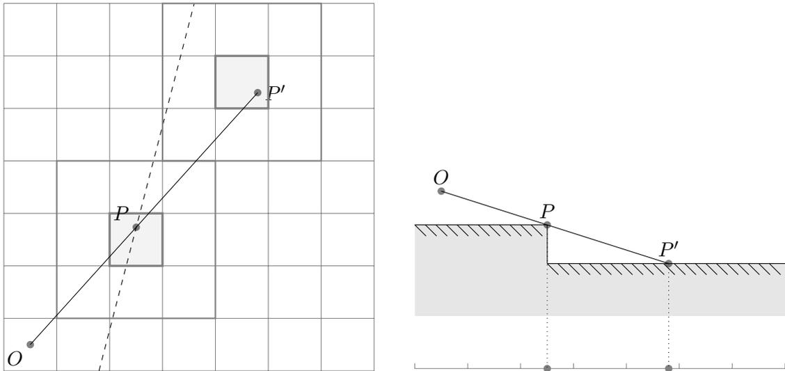
Figure 10.7: Left: A lidar beam originating in  $O$  touches the curb (dashed line) in  $P$  and hits the road below in  $P'$ .  $P$  and  $P'$  are entered in map cells (shaded) more than the 3x3 cell neighborhood away from each other. Right: A cross section of the situation with the sidewalk, the curb, and the road below (from left to right).
