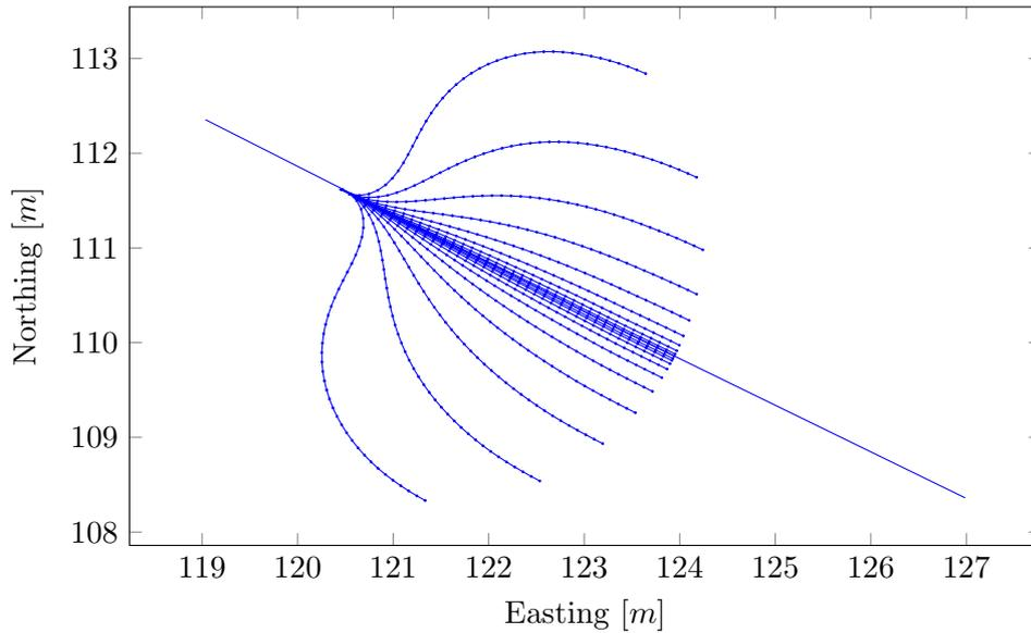
Figure 11.3: The tree formed by the application of candidate path offset functions with  $r = 0.8$  and  $i \in \{0, \dots, 9\}$  in both directions. Evaluation of candidates ends at a lookahead distance of 4 m.
