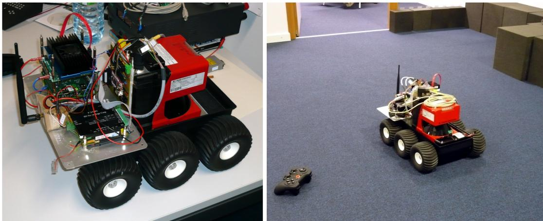
Figure 4.1: The SAMSMobil in its final pure-SAMS form. **Left:** The PC/104 board and DC/DC converter are mounted on the old battery compartment. The STM32 microcontroller board sits behind the laser range finder. **Right:** During a test run with the cordless gamepad.
