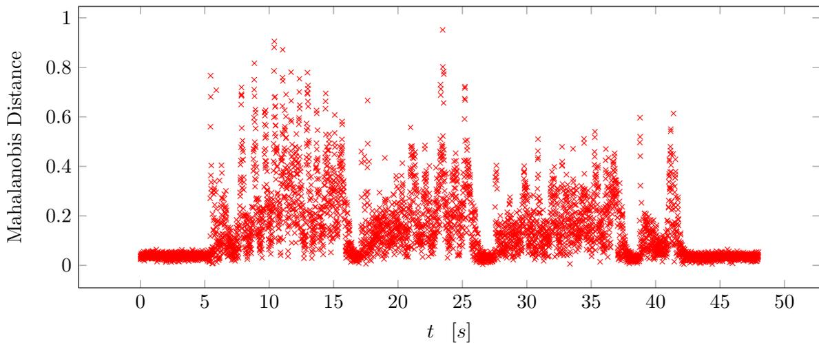
Figure 9.5: Mahalanobis distance of accelerometer measurements. The rear end of the robot was lifted a few centimeters and dropped several times. The resulting large accelerations violate the “at rest” assumption and are to be filtered out.
