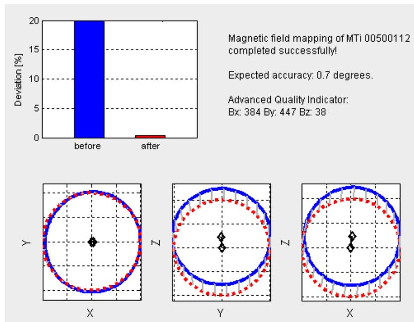
Figure 7.4: Screenshot of the 2D calibration report produced by the XSens Magnetic Field Mapper.
