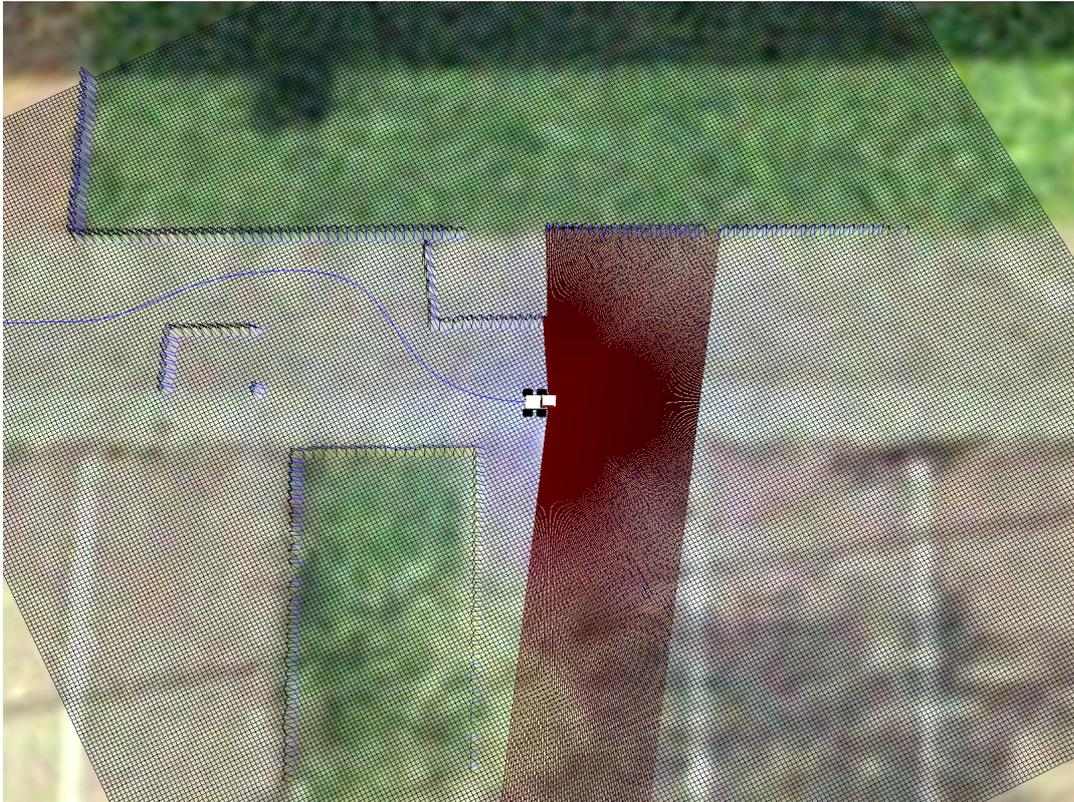
Figure 12.2: The robot after traversing the obstacle course in simulation. The local map is visualized as a wireframe surface.
