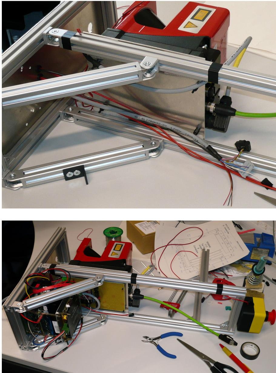
Figure 4.4: **Top:** The new cabling that connects the components above the base plate with those mounted in the chassis. **Bottom:** The PC/104 stack, solid state disk (SSD) and STM32 microcontroller board are mounted and the e-stop button connected.
