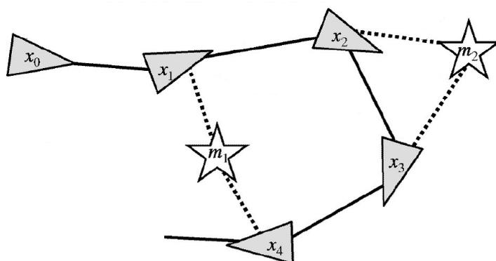
Figure 9.4: Constraint graph used by GraphSLAM (Image source: [Thrun et al. \(2005a\)](#); original annotations removed).
