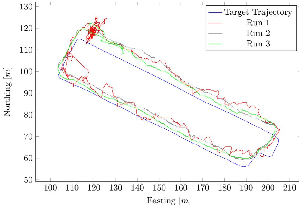
Figure 12.8: Raw GPS data from several test runs. The obvious quantization steps stem from the limited number of decimal digits transferred through the NMEA interface.
