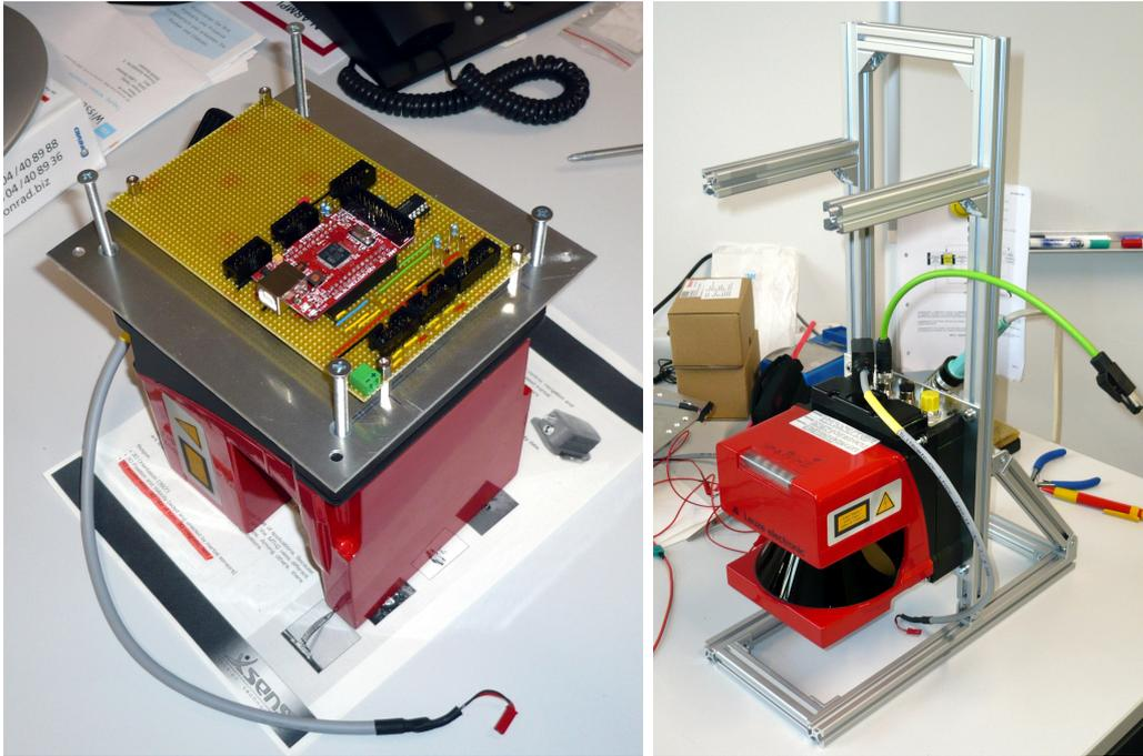
Figure 4.3: **Left:** The laser range finder is attached to an adapter plate which also holds the STM32 microcontroller board. **Right:** The same unit attached to the frame.
