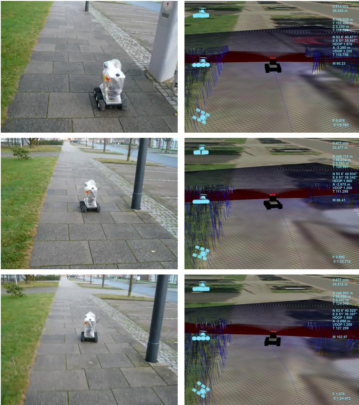
Figure 12.23: The SAMSMobil under autonomous control by the complete software stack in the 43 m test run: The bicycle and parking meter which had previously been a problem are passed successfully (top) and the lamp post is also avoided (middle and bottom).
