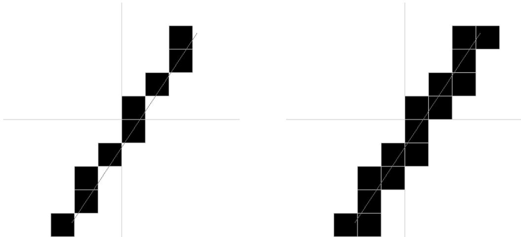
Figure 11.5: Bresenham line (left) vs. supercover line (right). The Bresenham line is visually pleasant but does not activate some cells although the straight line intersects them.
