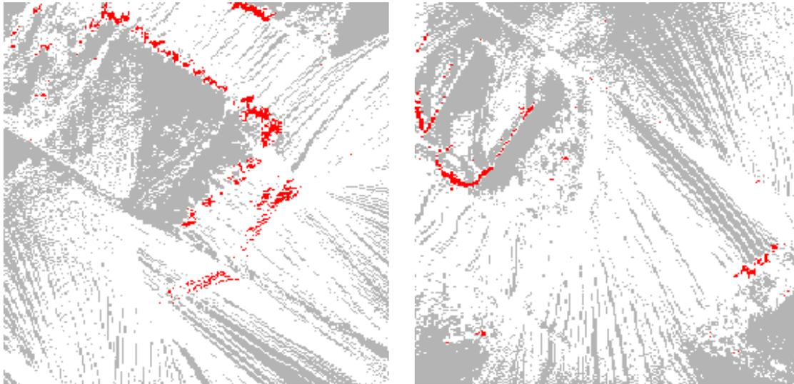
(a) Part of the ramp from the sidewalk (top) onto the road (bottom) is incorrectly detected as obstacles.
