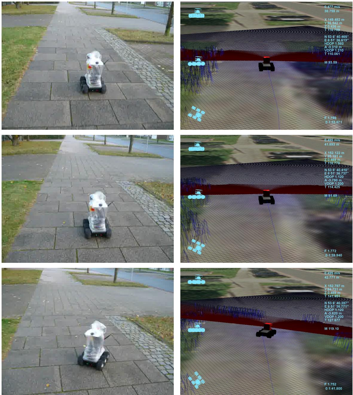
Figure 12.24: The SAMSMobil under autonomous control by the complete software stack in the 43m test run: The robot drives nicely centered on the sidewalk (top) but classifies the driveway as an obstacle (middle), veers to the side and blows the motor controller fuse (bottom).
