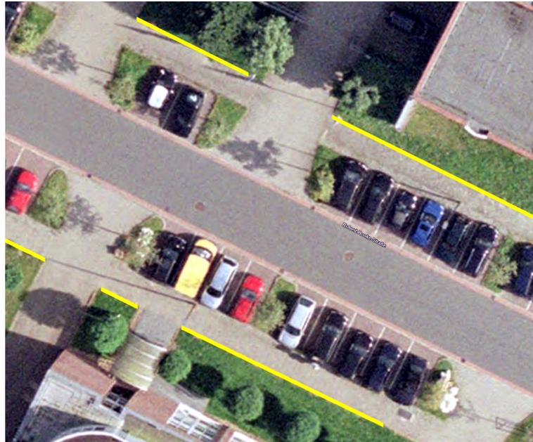
Figure 9.7: Part of the left hand side path boundary map (thick yellow line segments) for our test track in Google Earth.
