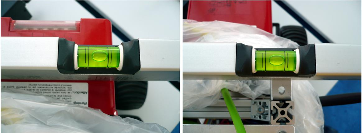
Figure 7.5: A level on top of the laser range finder case (left) and on the IMU/stereocamera head mounts (right). Up to the precision of the level the y-orientation of the two should be identical.
