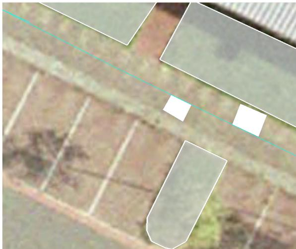
Figure 12.1: The obstacle course is defined as a set of polygons in Google Earth. To get past the two solid white obstacles, the planner needs to apply multiple different offset functions.
