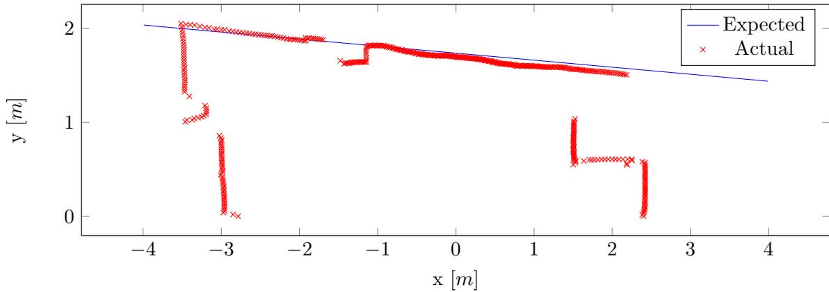
Figure 10.10: Expected ground plane intersection vs. actual laser range scan endpoints in an indoor setting. The plot shows the scan plane.
