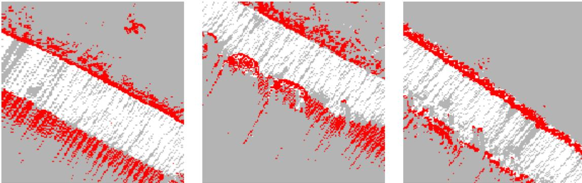
(a) GEM successfully detects the patch of grass (above) and the curb (below the path) as obstacles.
