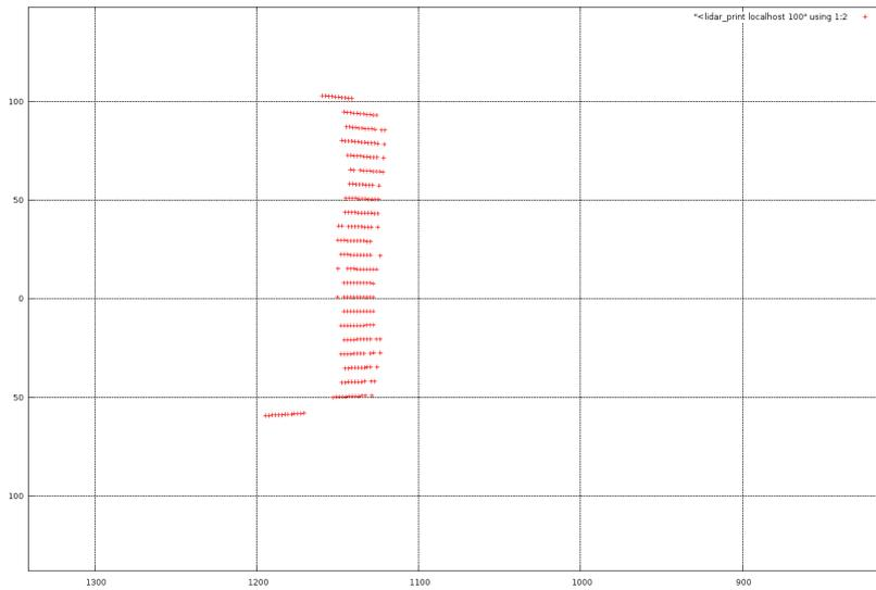
Figure 7.2: The surface of the calibration object as seen by the laser range finder (100 consecutive scans)
