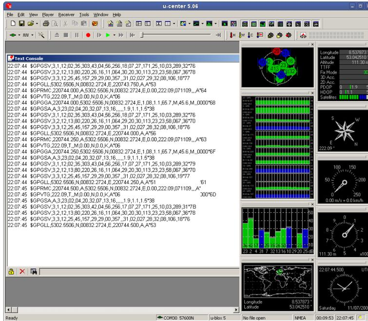
Figure 6.4: Screenshot of *u-center* showing NMEA output along with the visualized GPS data.
