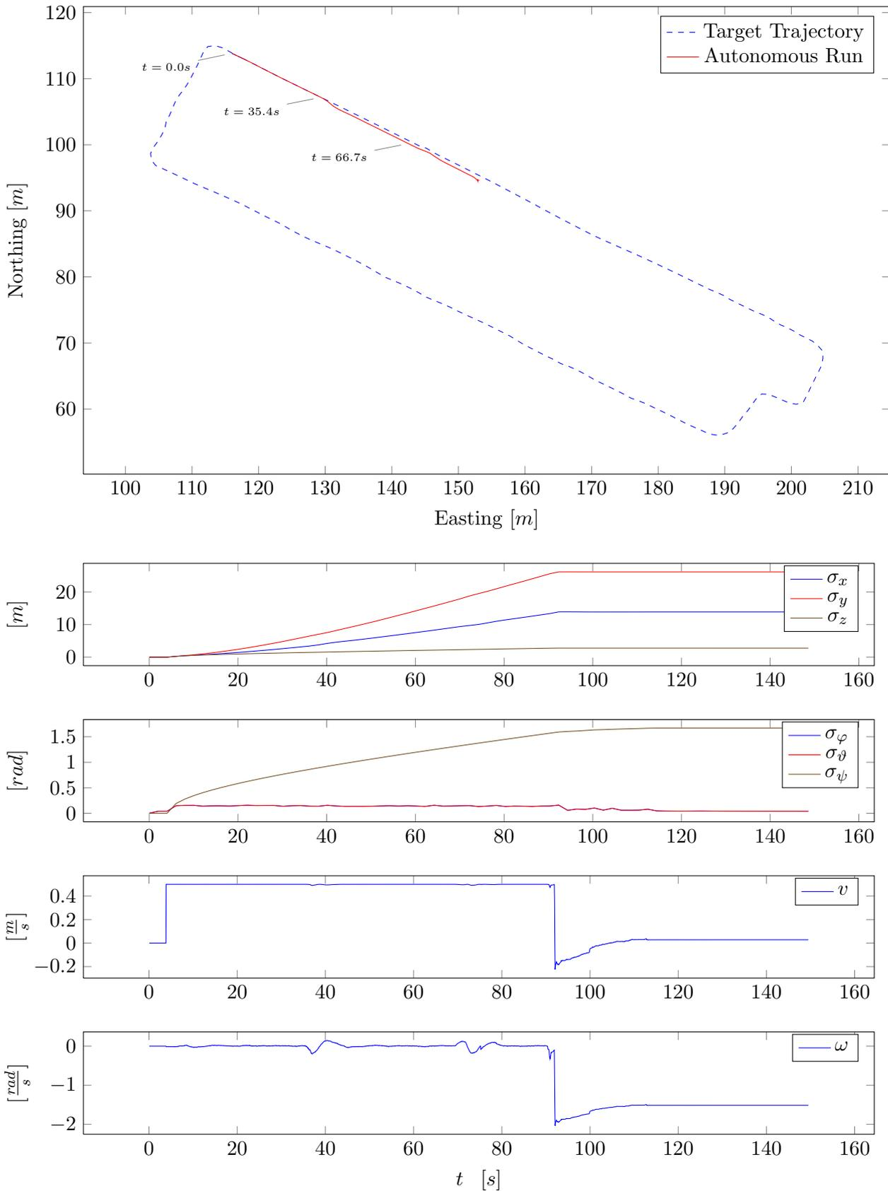
Figure 12.21: UKF position estimates and control commands from the 43m autonomous run.
