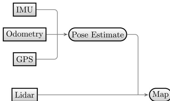
Figure 6.6: Sensor data sources (rectangular) and some of the products derived from them (rounded).
