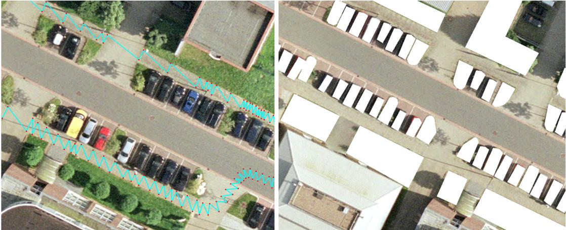
Figure 5.1: The zig-zag-line representing the goal path (left) and obstacle polygons for the simulation (right).
