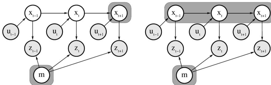
(a) Online SLAM (Image source: [Thrun et al. \(2005a\)](#)). (b) Full SLAM (Image source: [Thrun et al. \(2005a\)](#)).
