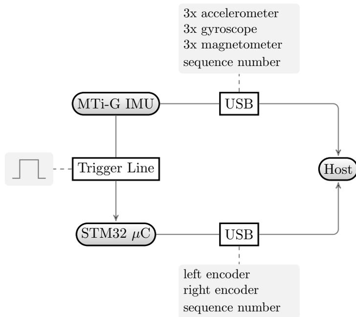
Figure 4.9: Overview of the IMU/odometry synchronization process. The MTi-G triggers the STM32. IMU and odometry messages are matched by their sequence numbers.
