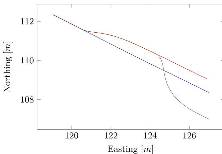
Figure 11.1: Consecutive application of two path offset functions with different parameters and in opposing directions.
