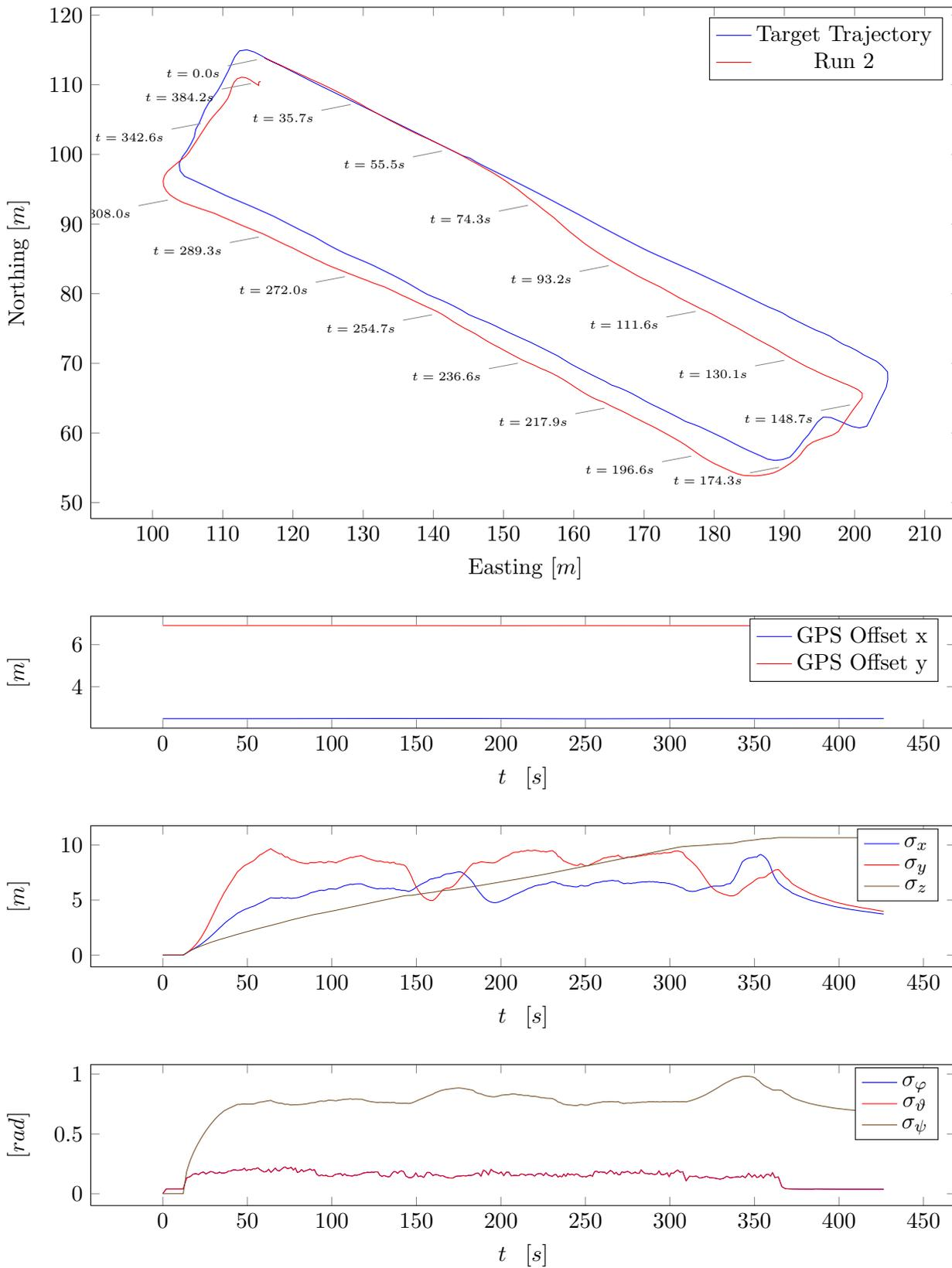
Figure 12.11: UKF position estimates with GPS measurements enabled. Here, too,  $\sigma_\phi$  and  $\sigma_\theta$  overlap.
