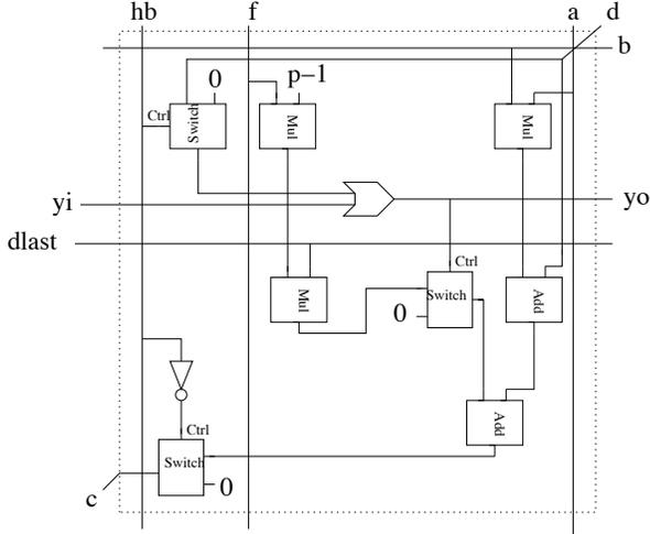
**Figure 2. Multiplier cell for  $GF(p^m)$**
