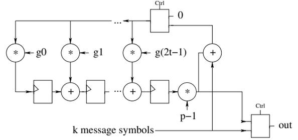
**Figure 3. LFSR Reed-Solomon Encoder for  $GF(p^m)$**
