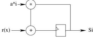
**Figure 5. Calculates  $S_i$  by evaluating  $r(x)$  with  $\alpha^i$**
