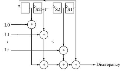
**Figure 6. Discrepancy calculator**
