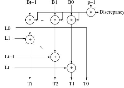
**Figure 7. Hardware for computing  $T(x) = \Lambda(x) - \text{discrepancy} \cdot X \cdot B(x)$**
