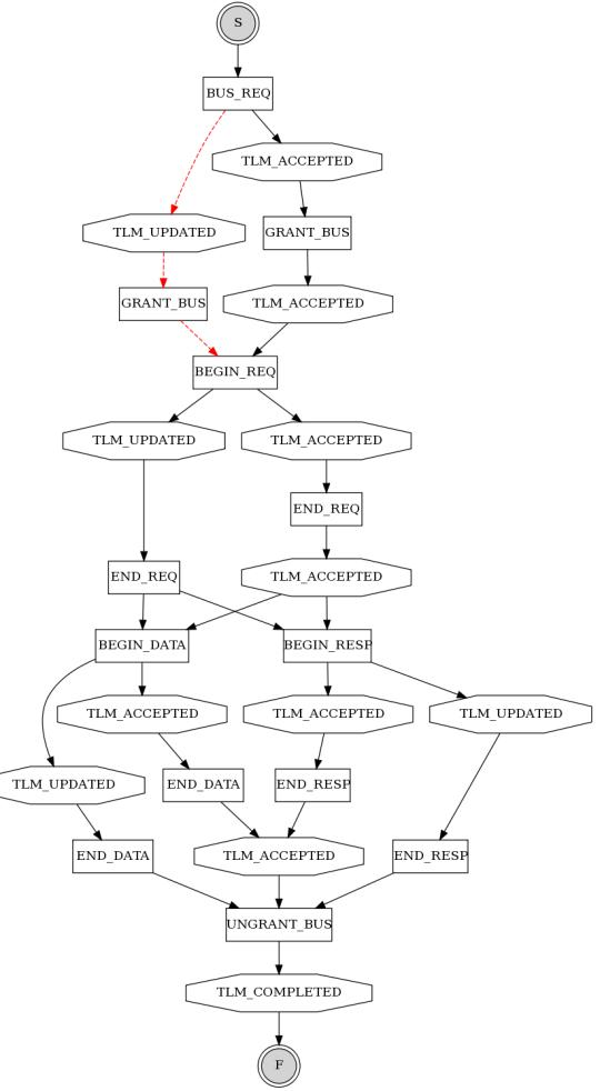
Fig. 6. Protocol sequence graph describing the protocol sequences for the write and read accesses
