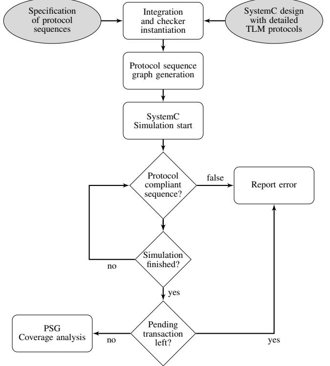
Fig. 2. Overall flow for protocol compliance checking
