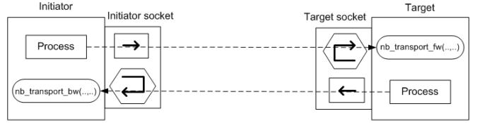
Fig. 1. OSCI TLM-2.0 connectivity between initiator and target
