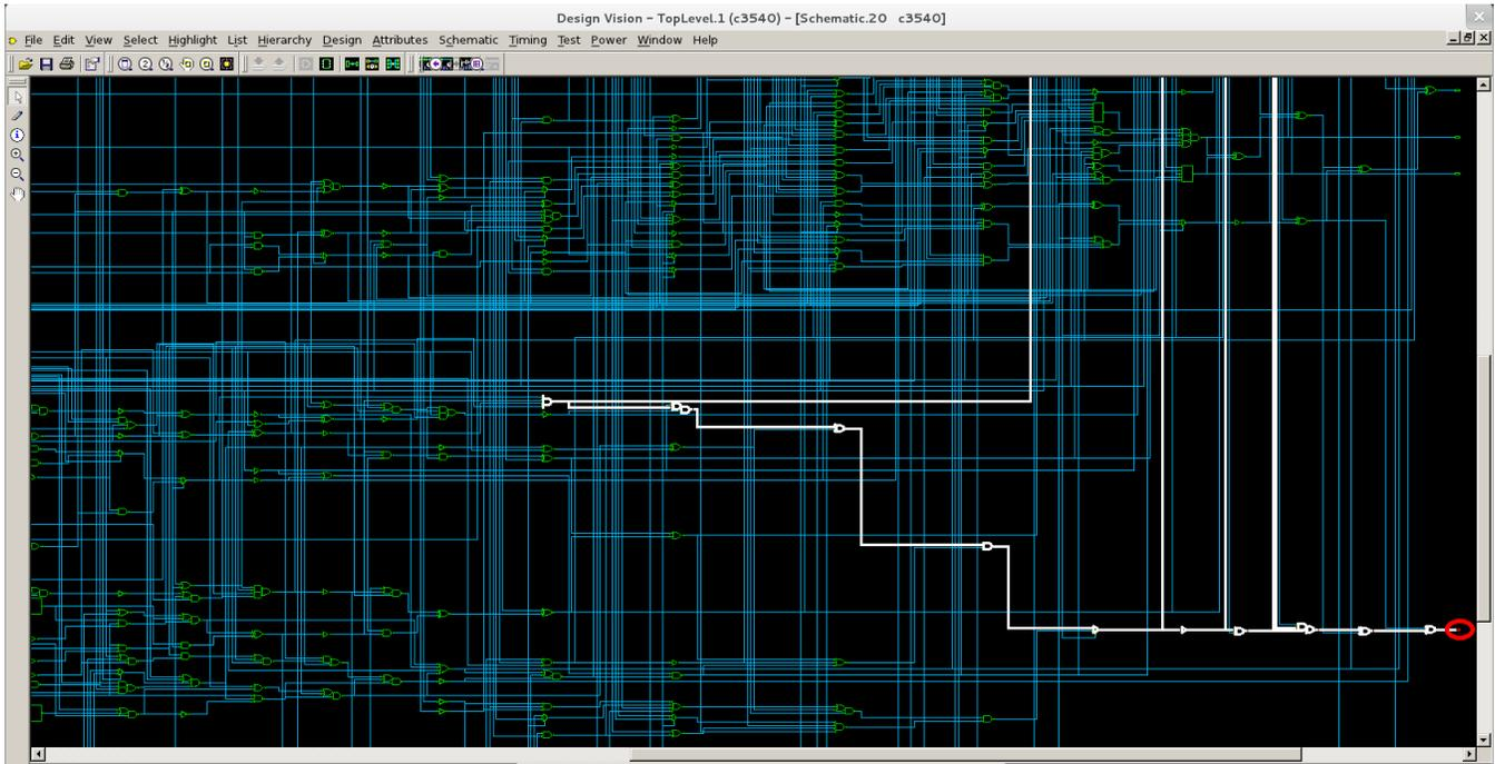
Fig. 2. Failing speedpath in circuit c3540
