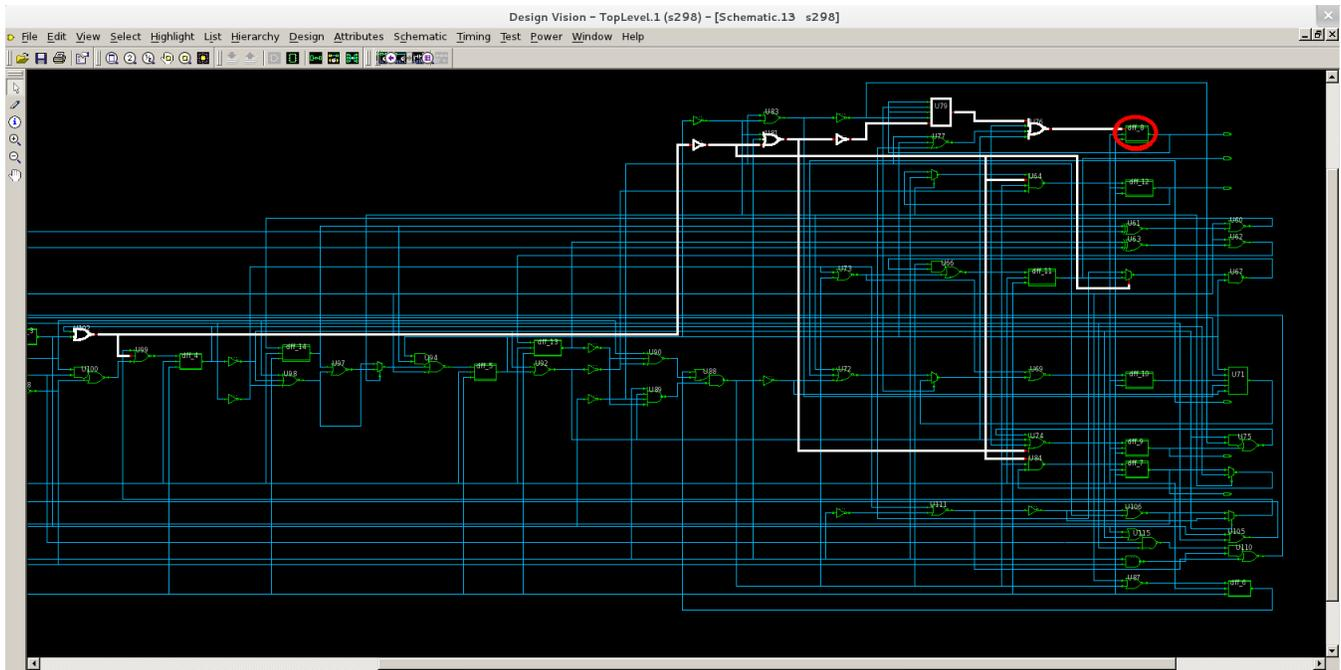
Fig. 3. Failing speedpath in circuit s298
