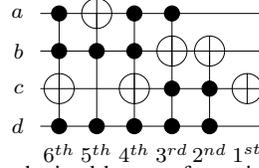
Fig. 1: Circuit obtained by transformation-based synthesis
