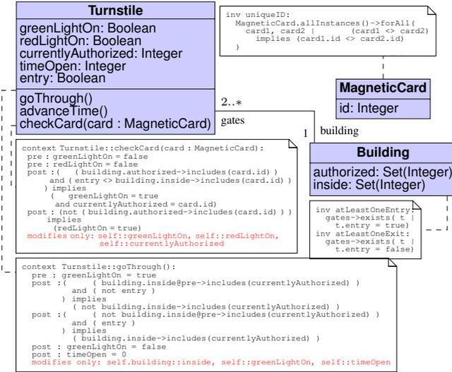
Figure 1: Class diagram of the access control system
