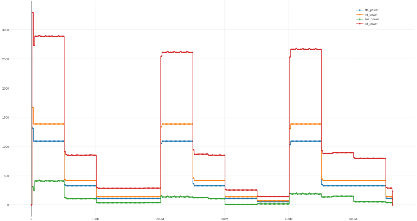
Fig. 9. Example power diagram of a concrete workload from scenario S3. It shows the static, internal, switching and total power consumed of all components at different simulation time steps.
