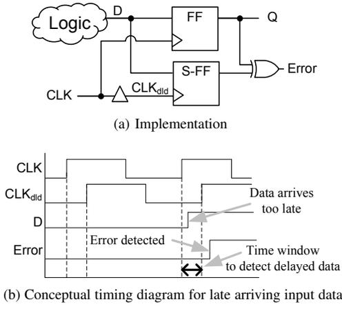
Fig. 1: Soft-Error sensing based on transition detection.
