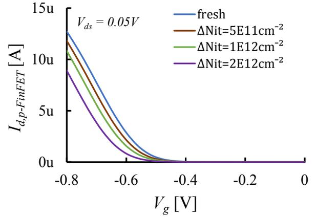
Fig. 3:  $I_d$  over  $V_{gs}$  for p-FinFET and NBTI-dependent increase of the threshold voltage.
