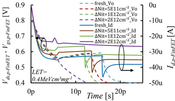
Fig. 9: p-FinFET  $I_d$  and  $V_{ds} - V_{gs}$  after heavy ion strike with  $LET = 0.4MeVcm^2mg^{-1}$  on n-FinFET before (blue) and after (brown, green, purple) incorporating NBTI-induced device degradation.
