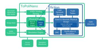
Fig. 7: Schematic view of ToPoliNano design flow and how *fic-tion*'s SMT-based exact physical design algorithm is available as a plug-in for ToPoliNano's place & route engine to generate optimal building blocks in the hierarchical layout process.
