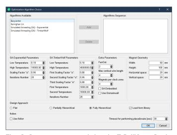
Fig. 5: Layout parameter window in ToPoliNano. In the top part the optimization algorithms, in the centre layout parameters, and in the bottom part the layout approach.
