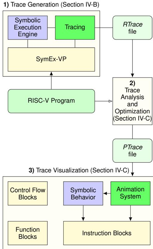
Fig. 1. Overview on the architecture of our proposed 3D visualization framework
