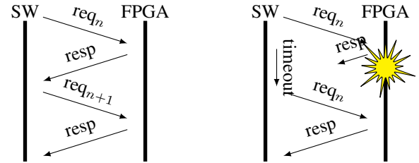
Fig. 4. Transaction-based processing and transaction-retry after a soft error in hardware. Figure reused from [4].
