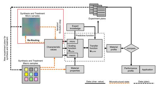
Fig. 2. Information flow of the high throughput approach [13]
