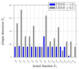
Fig. 5. Built and trained kernel functions for Transfer Function (using alloy 100Cr6 with 5 grid points) with two different level of certainty (TRSH)
