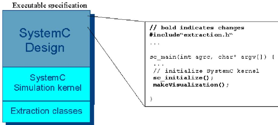
Figure 4: Connection to the simulation kernel of SystemC
