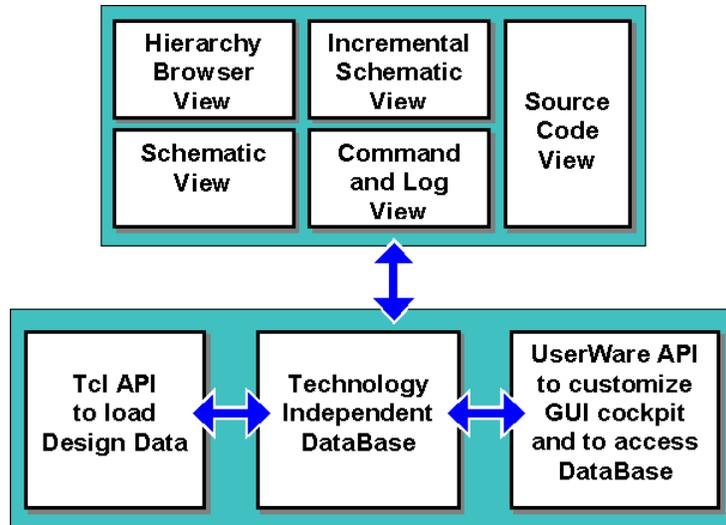
Figure 2: Architecture of Concept Engineering's customizable GUI cockpit
