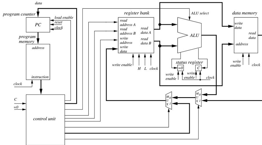
Figure 1. Structure of the RISC CPU including data and instruction memory
