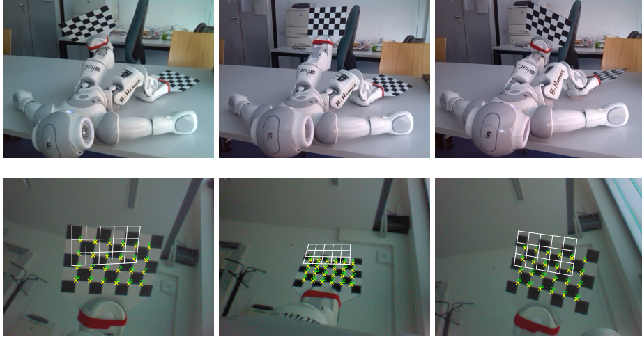
Fig. 3. Some snapshots taken during a calibration experiment. The upper images show different joint angle configurations, whereas the lower figures depict the corresponding points of view of the lower camera.
