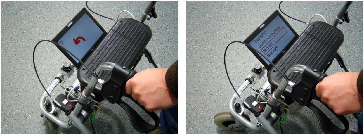
Fig. 3. The Navigation Assistant. The left picture shows the arrow guiding the user to the target location. The right picture shows the menu to select a new target location. The selection is done by moving the iWalker.
