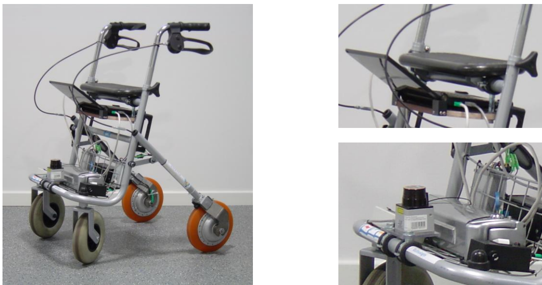
Fig. 1. The iWalker with electrically breakable rear wheels, a netbook, and a laser range sensor. The netbook is mounted below the seat (upper right picture, also cf. Fig. 3). The Hokuyo laser range sensor is installed at the front (lower right picture).
