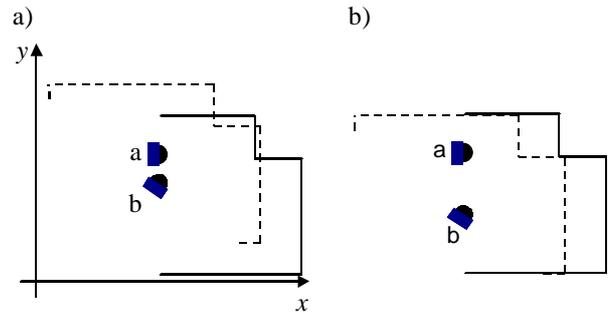
**Figure 7:** Correction of the first translational shift
