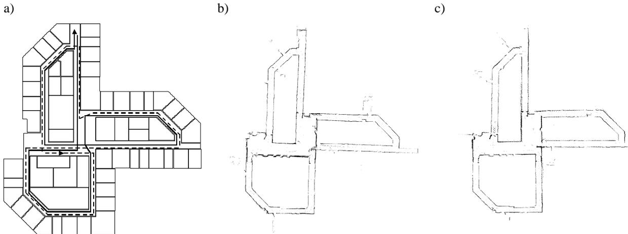
**Figure 10:** Two maps of the same environment generated on different routes
