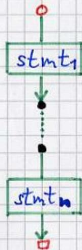
falls  $\text{stmt} = \text{begin stmt}_1; \dots; \text{stmt}_n \text{ end}$
