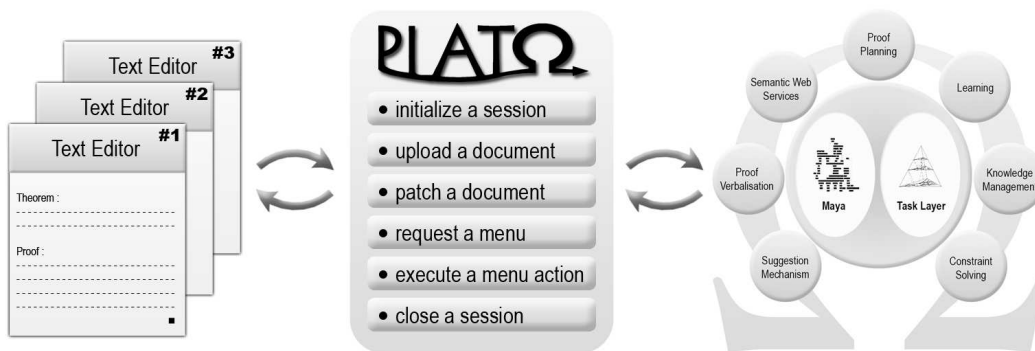
Figure 1. Architecture of integration of the text-editor and the \Omega MEGA via the mediator PLAT \Omega .
