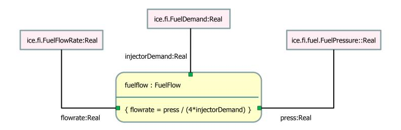
Relation of fuel flowrate to FuelDemand and FuelPressure value properties (Source: OMG SysML v1.2)
