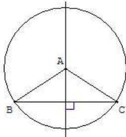
For instance, in the constraint (isosceles  $ABC$ ) which means  $AB = AC$ , to build the point  $A$ , we build the perpendicular bisector of  $[BC]$ , but to build the point  $B$  we build the circle of center  $A$  with radius  $[AC]$ .
