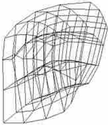
Figure 4.14: In one of our customers' VR lab, the distortion of the Ascension's field is about 50 cm max. The volume measured is about  $2 \times 2 \times 1 \text{ m}^3$ , with a long-range transmitter positioned 2 m above the floor and 3 m below the ceiling.
