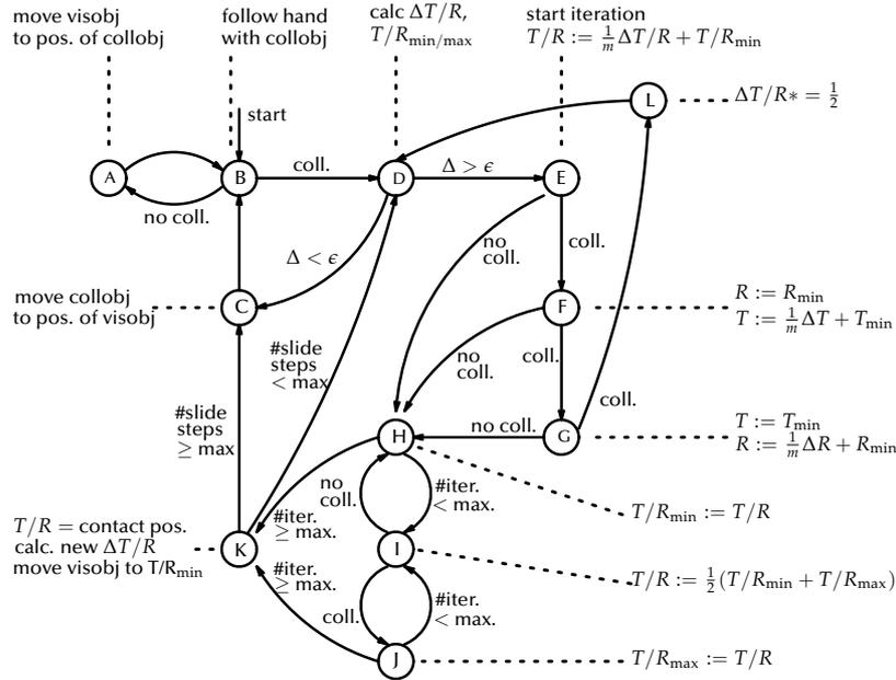
Figure 4.43: The main loop of the sliding simulation is a finite state machine.
