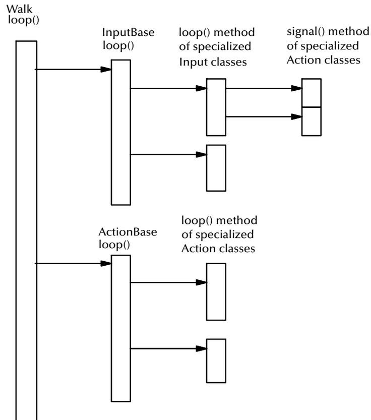
Figure 2.14: Basic sequence diagram of the interaction manager.
