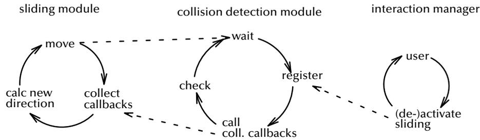
Figure 4.42: The physically-based simulation module for sliding runs concurrently to the other two main loops of the collision detection module and the interaction manager. Dashed arrows mark rendezvous points.
