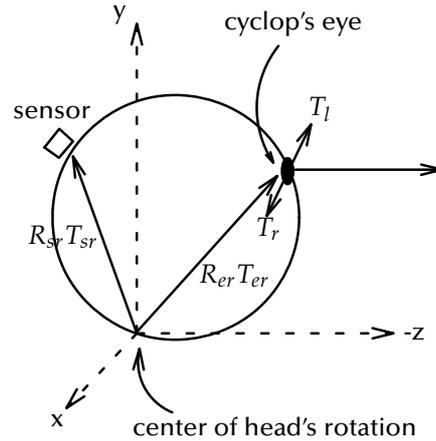
Figure 4.36: Transformations associated with the head model.
