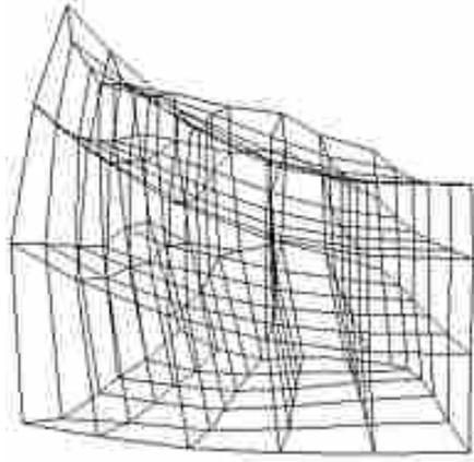
Figure 4.10: Visualization of the distortion of the field: the nodes of the lattice are measured points of a uniform lattice. The discrepancy can be as much as 40–50 cm (15–20 in).
