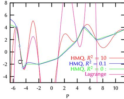
Figure 4.19: 1D examples of HMQ interpolation functions through 10 points with various  $R^2$  parameters. For  $R^2 = 0$  the function is piecewise linear. The Lagrange interpolant exposes fatal oscillations.
