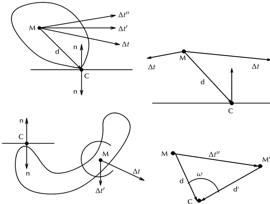
Figure 4.44: With one contact point, calculation of the direction of the new translational velocity is the same whether or not the contact normal points to the “right” side.
