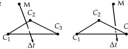
Figure 4.49: With 3-point contacts, 2 different situations must be distinguished: when looking along the old translational velocity,  $M$  can be “inside” the convex polygon spanned by  $C_1, C_2, C_3$  or “outside”.
