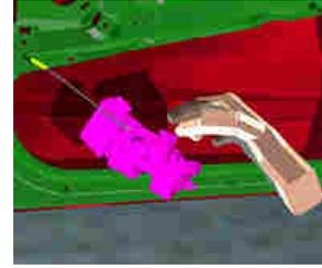
Figure 5.10: The object-on-the-lead paradigm allows to verify assembly. The object is not linked rigidly to the hand.
