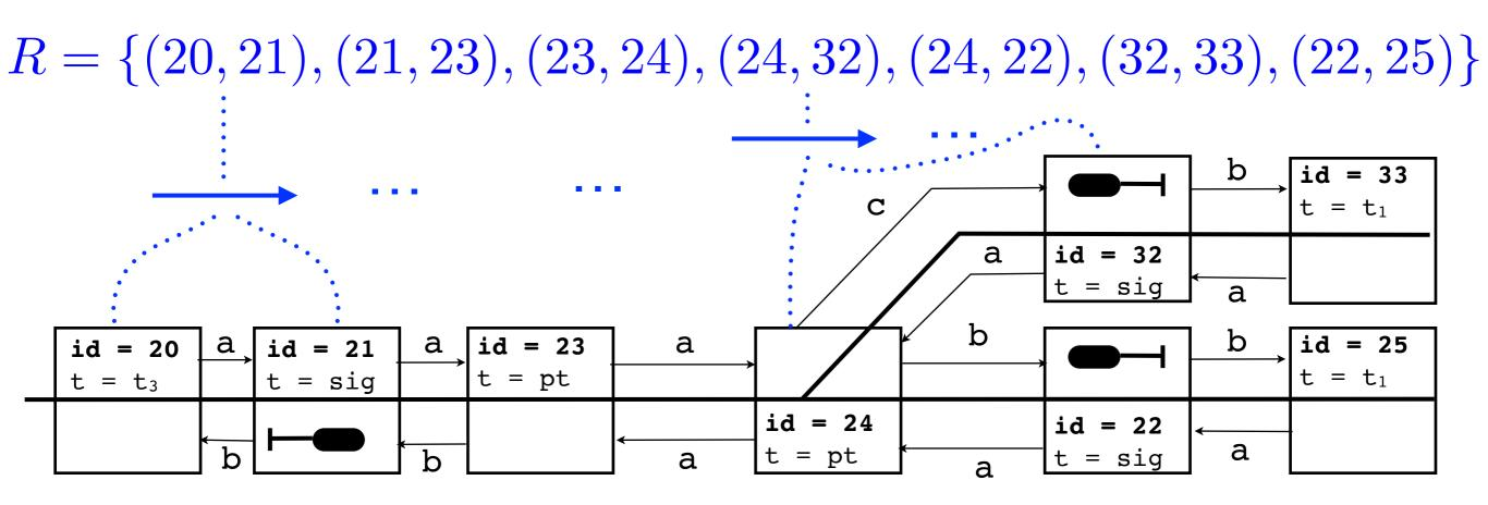
**Sub-model.** Sub-graph of element instances from one entry element to all exit elements reachable in driving direction
