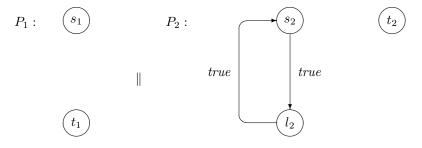
Process  $P_1$  can never execute any transition (not even a transition to terminate), so it is always blocked. Process  $P_2$  executes its loop infinitely, therefore, the complete program is deadlock free. We choose the assertion networks as below:
