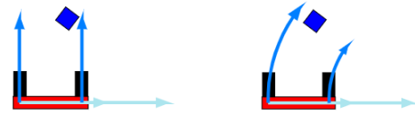
Figure 2: The simulated robot with two out of the four cardinal DoFs (left) and two adaptive DoFs (right)
