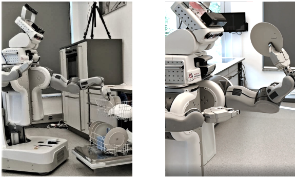
Fig. 5. Qualitative evaluation (left): Robot empties the dishwasher, based on RGB data fused with the knowledge of the dishwasher compartments (as support plane); Detecting object in Hand with gripper pose as prior knowledge (right) - quantitative evaluation against RGB and RGB-D data. The whole task can be seen in the accompanying video.
