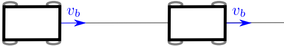
Figure 3: Vehicle driving a straight line. The velocity is not observable with the forward velocity prior.
