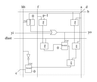
Figure 2. Multiplier cell for  $GF(p^m)$
