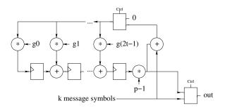
Figure 3. LFSR Reed-Solomon Encoder for  $GF(p^m)$
