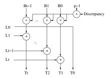
Figure 7. Hardware for computing  $T(x) = \Lambda(x) - discrepancy \cdot X \cdot B(x)$
