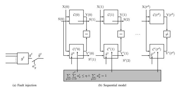
Figure 2. Sequential model with fault injection logic
