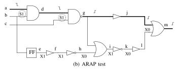
Fig. 1. Tests for path a - d - g - j - m
