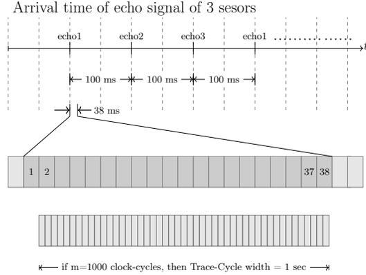
Fig. 5: Sensor data in a trace-cycle
