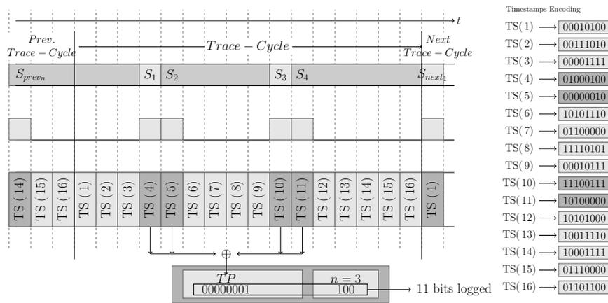
Fig. 1: An intermediate trace-cycle, with its respective timeprint
