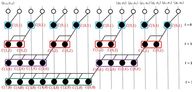
Fig. 7. The complexity calculations for a 16-bit Ladner-Fischer adder
