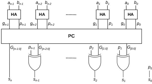
Fig. 1. The general structure of a prefix adder
