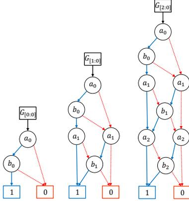
Fig. 6. The BDDs for  $G_{[0:0]}$ ,  $G_{[1:0]}$ , and  $G_{[2:0]}$
