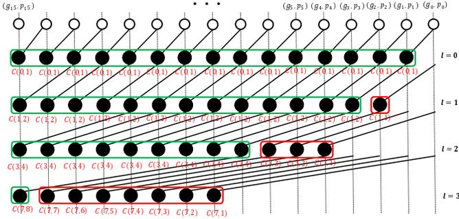
Fig. 8. The complexity calculations for a 16-bit Kogge-Stone adder
