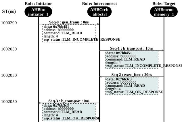
Figure 4: UML diagram of SoCRocket-VP’s LT transaction.
