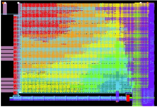
Fig. 6: IR-drop contour by commercial tool
