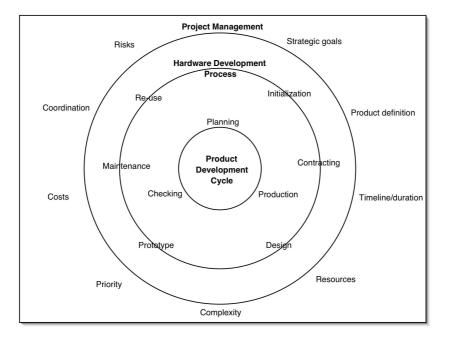
Figure 2: Three Layer Model of Hardware Engineering
