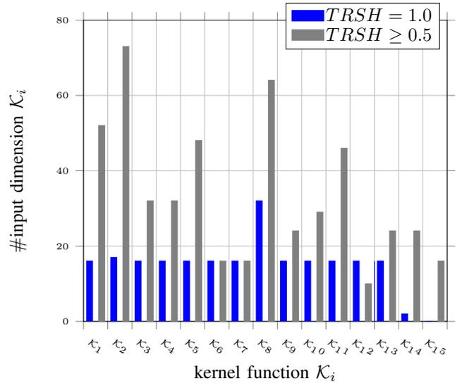
Fig. 5. Built and trained kernel functions for Transfer Function (using alloy 100Cr6 with 5 grid points) with two different level of certainty (TRSH)
