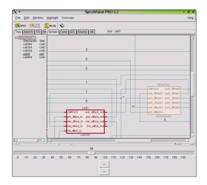
Figure 7: System level view of arbiter with simulation data
