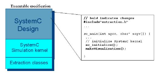
Figure 4: Connection to the simulation kernel of SystemC
