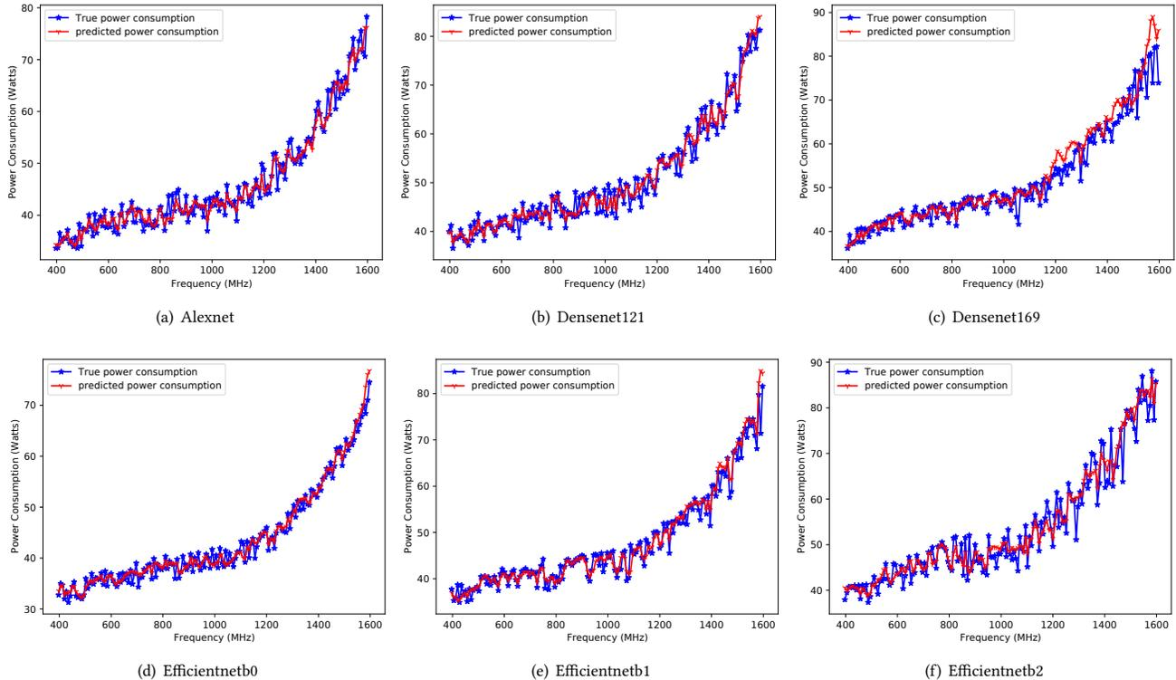
**Figure 5: Comparison of predicted and real power consumption for six different CNNs for frequencies between 397MHz and 1590MHz on the Nvidia V100S GPGPU.**
