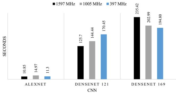
(b) Run-time of various CNNs for different frequencies inferencing on Nvidia V100S
