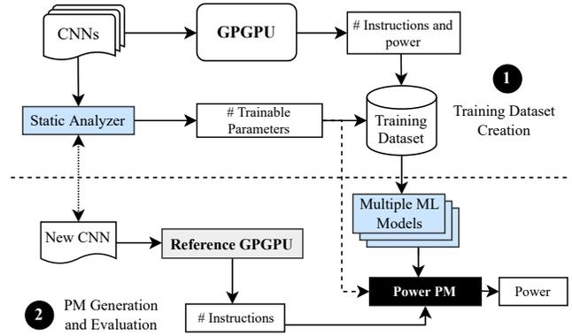
**Figure 2: DFS-based power estimation methodology.**
